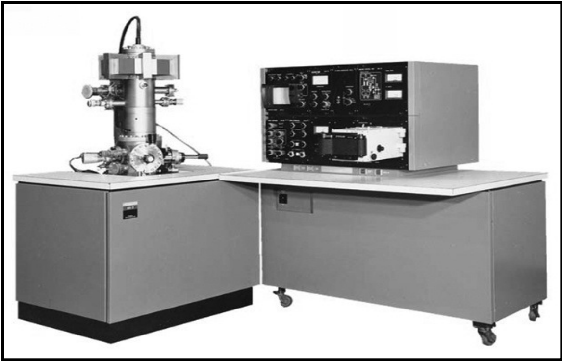
Figure 3.9 Basic model of field emission scanning electron microscope (FESEM) [39]
