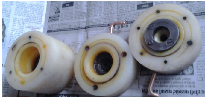
Figure 1.3 Fixture in three parts
