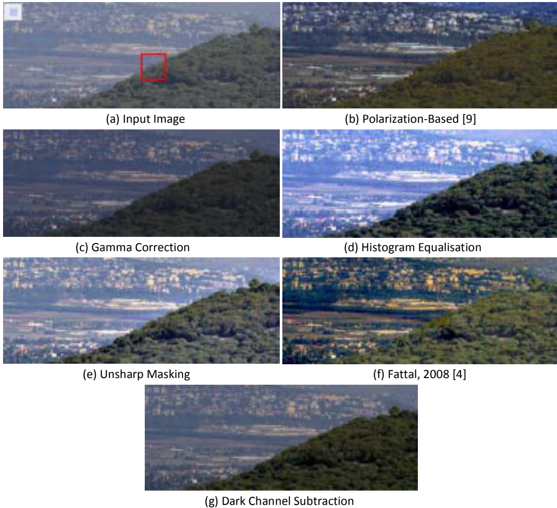
Figure 3.1.: Comparison of computed images from the same input image created with different dehazing techniques. [4]
