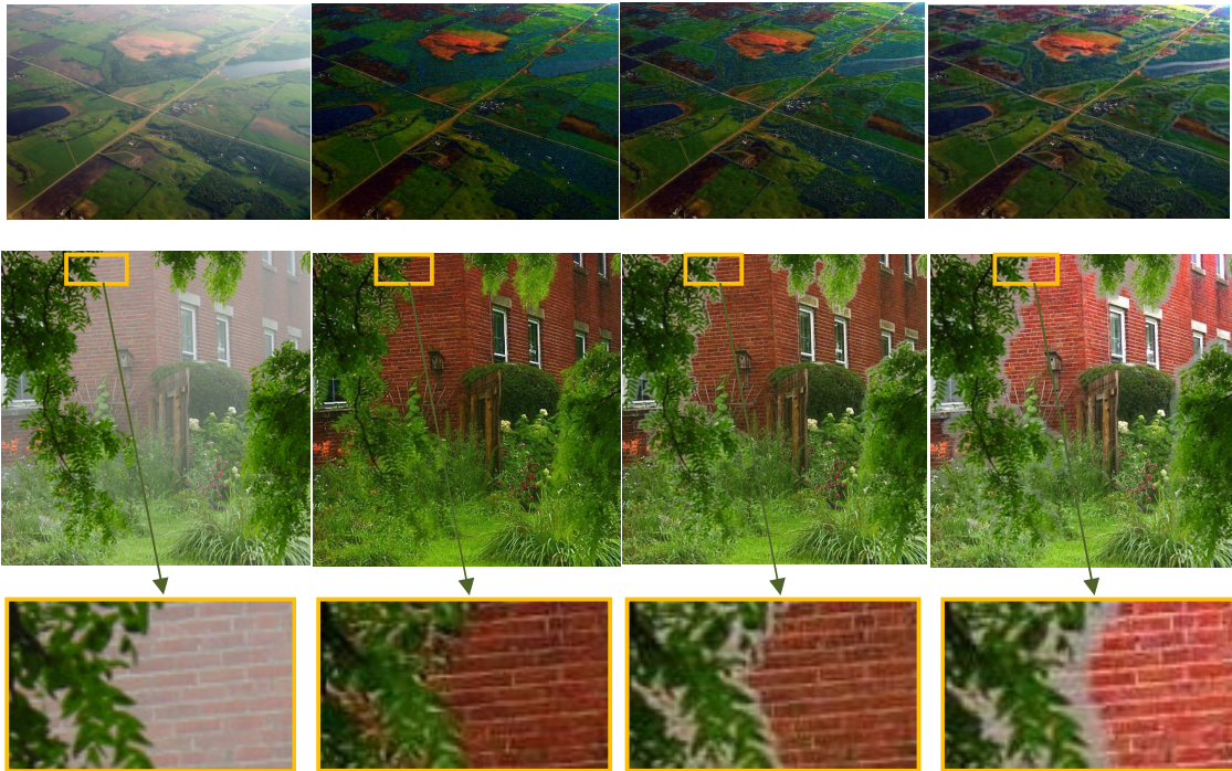
Figure.: 4.9 Recovering images using different patch sizes (after refining). (a) Input hazy images. (b) Using 3 x 3 patches. (c) Using 7x7 patches. (d) Using 15x15 patches.
