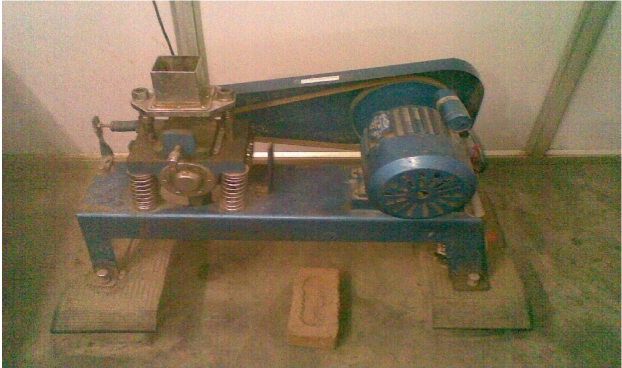
Photo: 3 Vibration machine to shaking the mortar filled mould.
