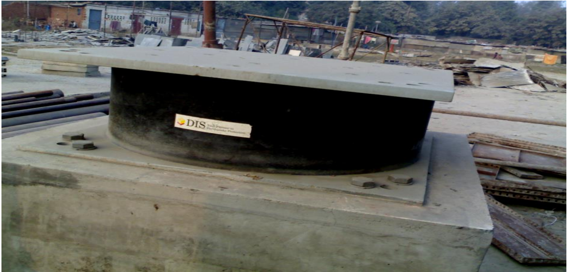
A Prototype View of Lead Rubber Bearing Used in GTB Hospital Base-Isolated Building at Delhi Dilshad Garden
