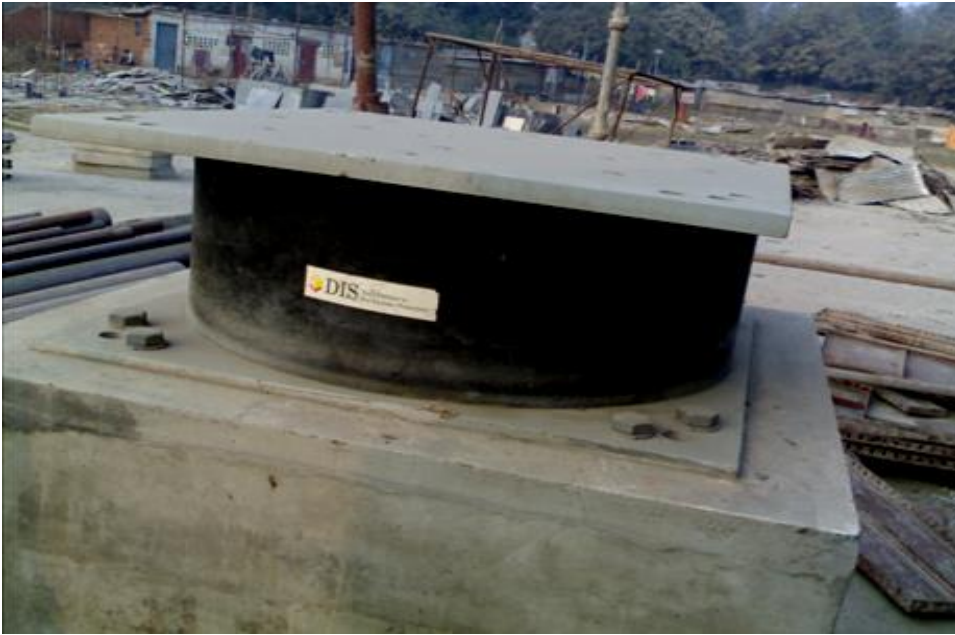
A PROTOTYPE VIEW OF RUBBER BEARING USED IN GTB BASE ISOLATED HOSPITAL ,ELHI
