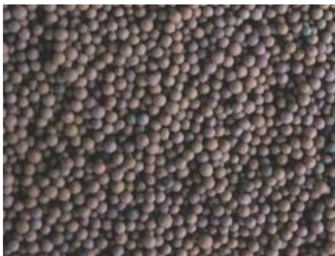
Figure 4.2: BIOLITE media used in BIOFOR
