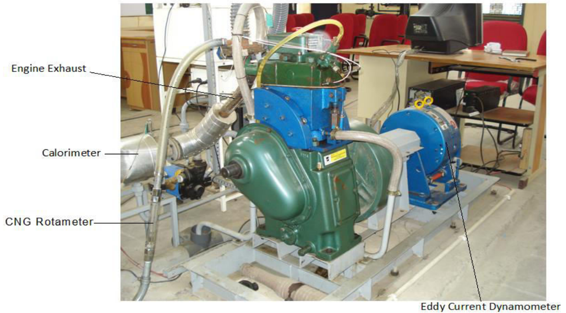
Figure 4.3 a Actual Diesel-CNG VCR Engine Test Setup
