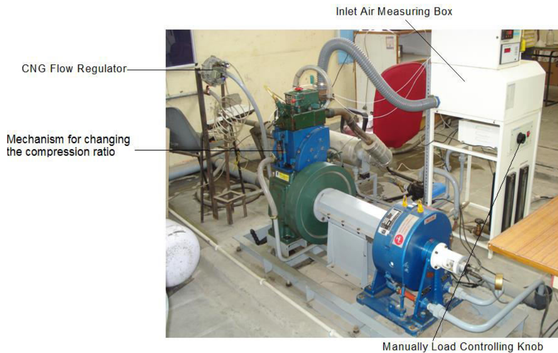
Figure 4.3 b: Actual Diesel-CNG VCR Engine Test Setup
