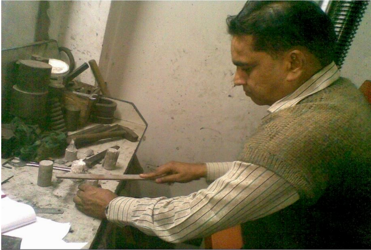
Photo: 5 Making plane the surface of specimen with help of grinder
