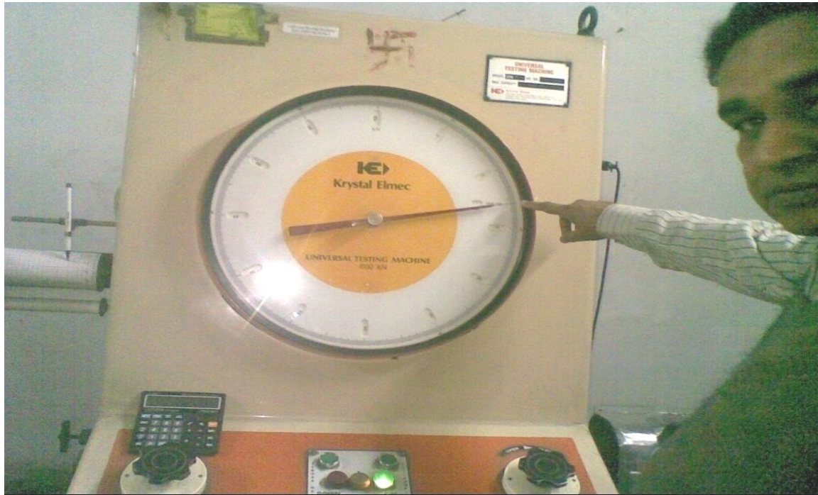
Photo: 8 Observation of uniaxial compression machine at failure of specimen .
