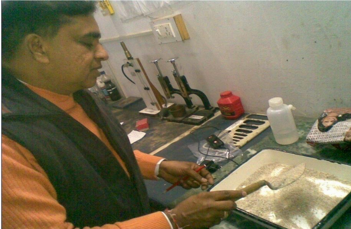
Photo: 1 Mixing of standard sand with 43 grade OPC cement.
