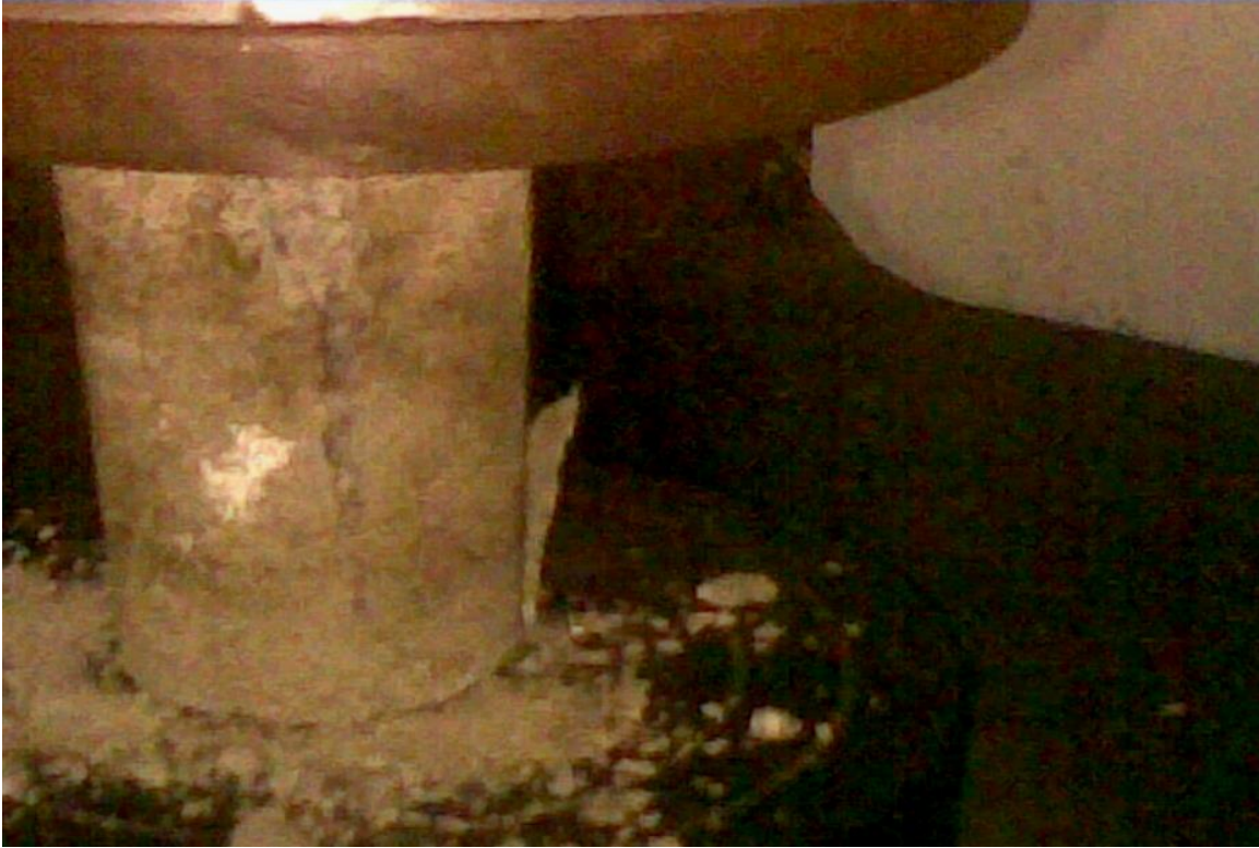
Photo: 9 Specimen at failure.
