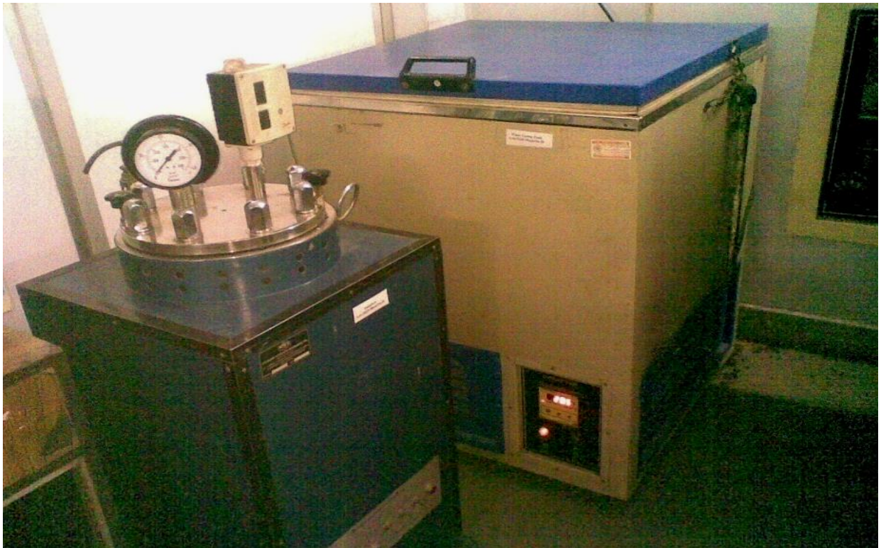
Photo:4 Photograph of curing tank in which specimen were laid for curing.
