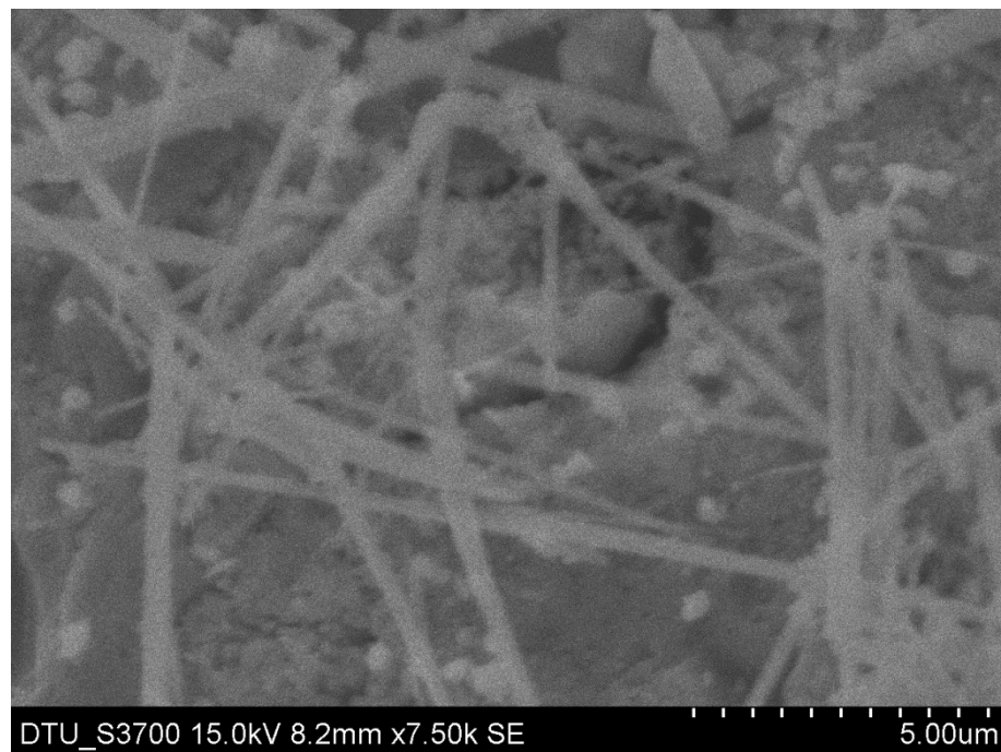
Figure 5.1(c): SEM micrograph of sample PbSe at 4h
