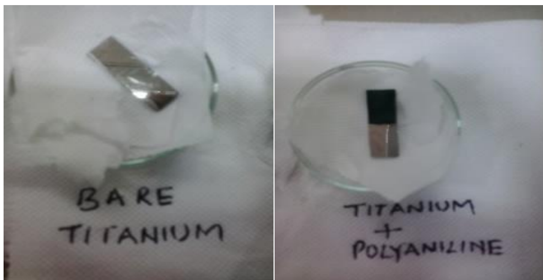
Figure 2.7: Photograph of Titanium film before and after deposition
