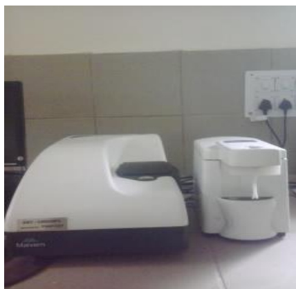
Figure 2.5: Photograph of Dynamic Light Scattering instrument (Zetasizer) at BECPRL-NPL
