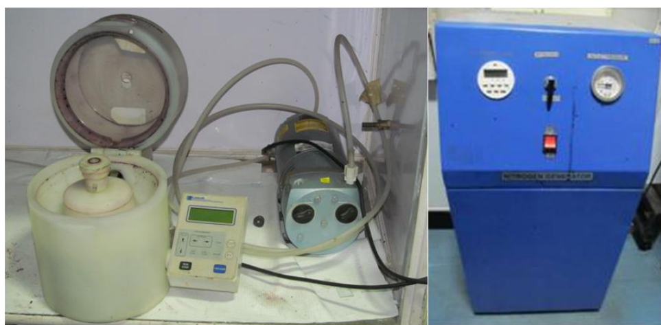
Figure 3.9: Digital spin coater used at NPL, Delhi
