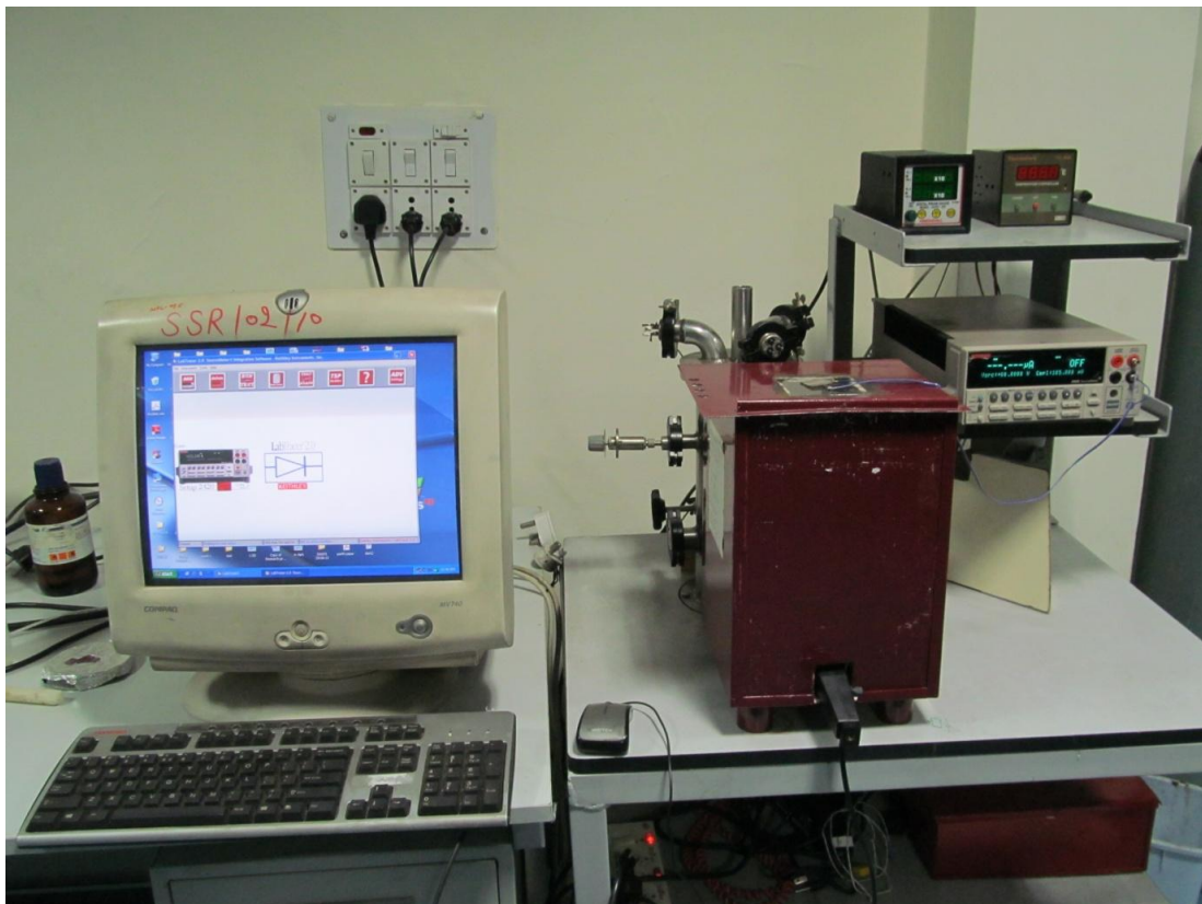
Figure 4.6: Set-up for J-V characterization of the device.
