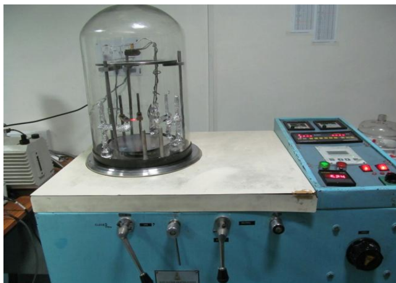
Figure 4.4: Thermal Evaporation Unit at NPL, New Delhi
