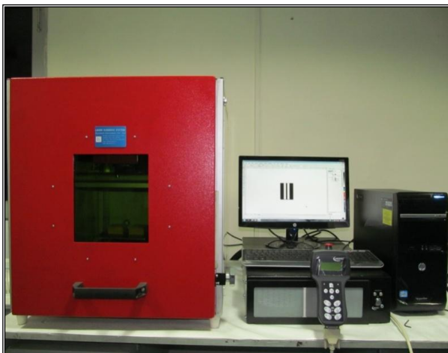
Figure 4.1: Laser Scribing Unit at NPL, Delhi
