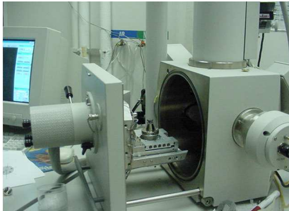
SEM opened sample chamber (10)
