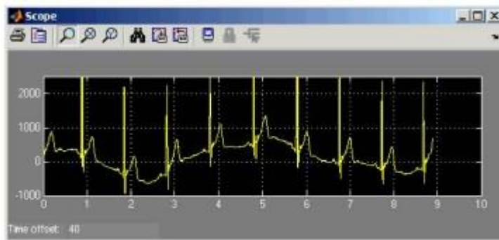
Fig4.3 This simulink Scope shows an acquired ECG signal with a sampling frequency of 1200 Hz
