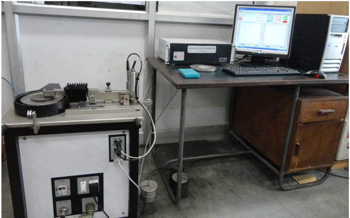
Figure 3.8- Wear and friction monitor machine for pin on disc test
