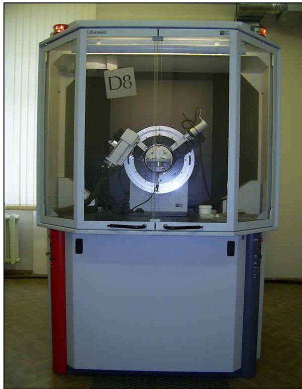
Figure 3.13-X-Ray diffractometer in DTU, Delhi
