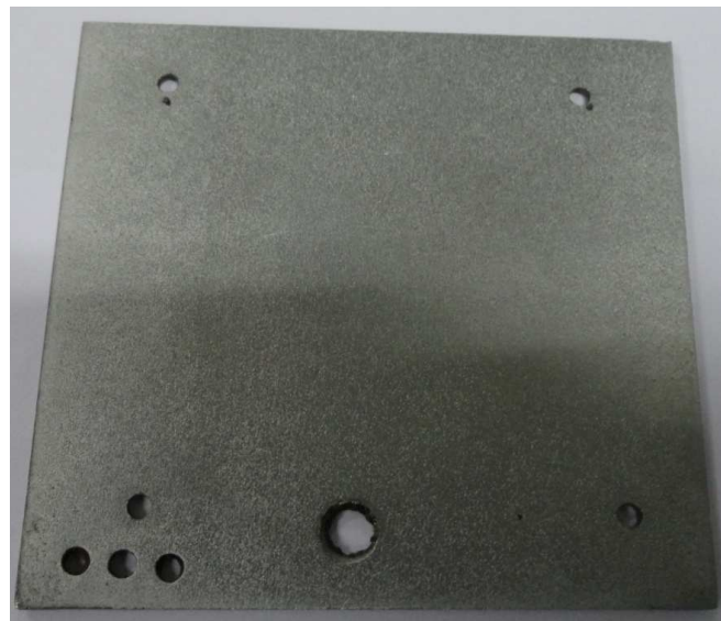
Figure 3.9 Hard Chrome coating before wear test
