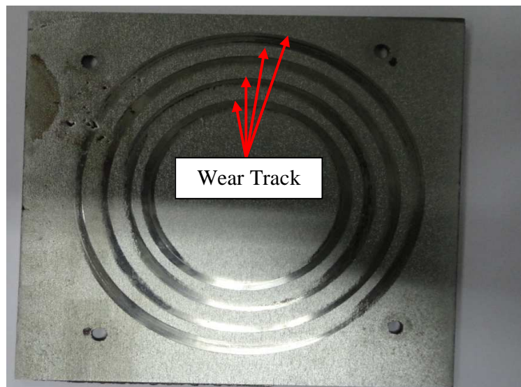
Figure 3.11 - Hard Chrome coating after wear test
