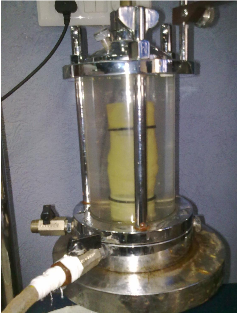
Figure C: Tri-axial testing (picture at the failure of sample)
