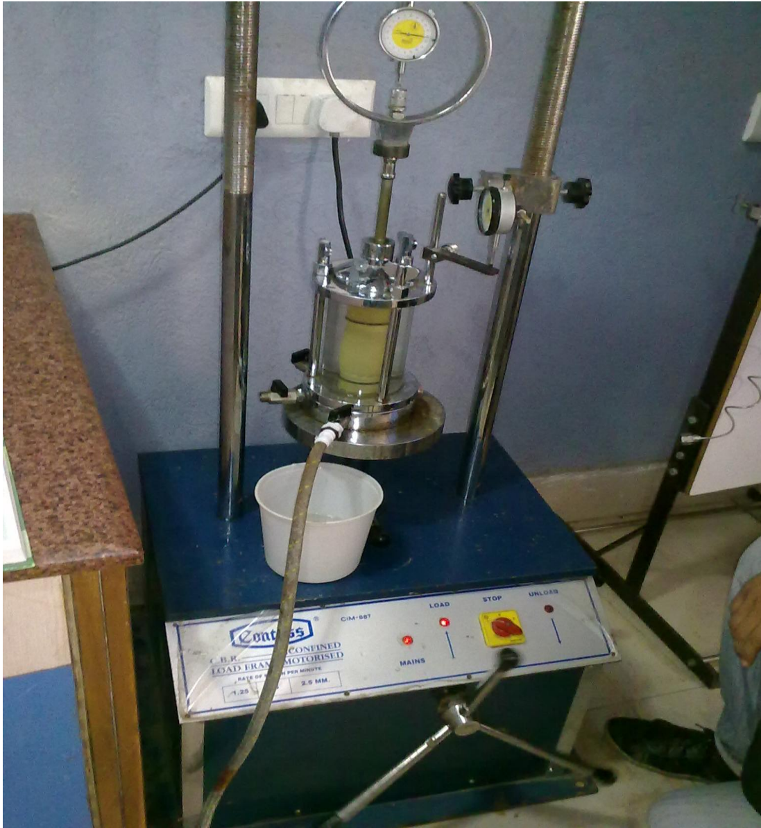
Figure B: Tri-axial testing (during loading)
