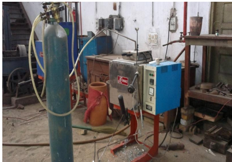
Fig. 3.3 Melting arrangement facility of developed Mg-alloys at CSIR-NML
