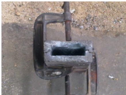
Figure 3.1 Schematic diagram of the mould used for magnesium alloy castings
