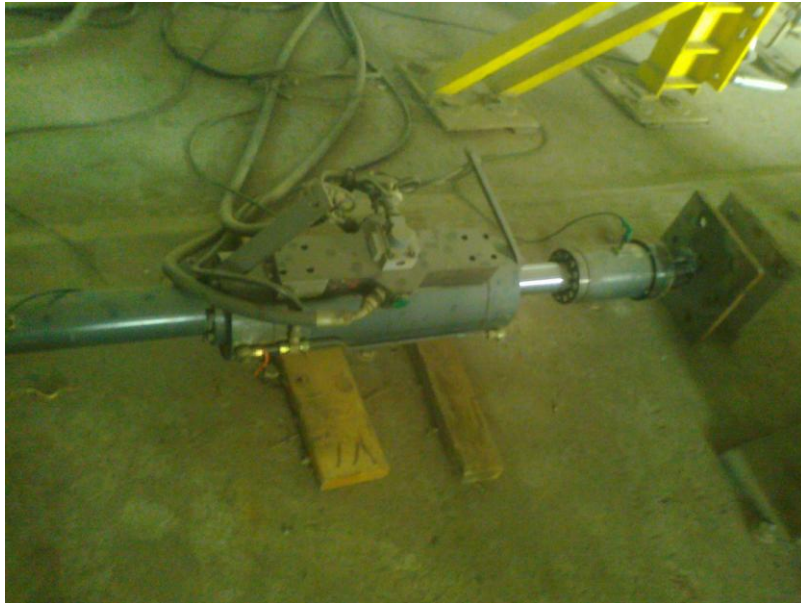
Fig.3.19 (b): Actuator (displacement based) by INSTRON
