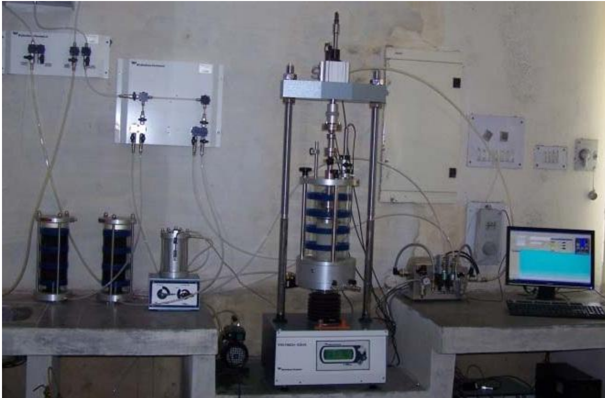
Fig.3.25. Cyclic Triaxial System at the Department of Earthquake Engineering, IIT Roorkee.
