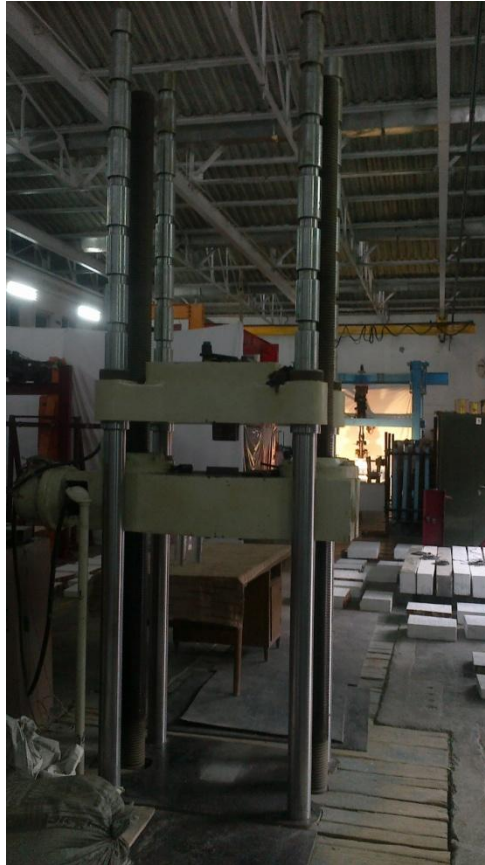
Fig.4.2: 2000 kN Universal Testing Machine( Tinious Olsen,USA,)
