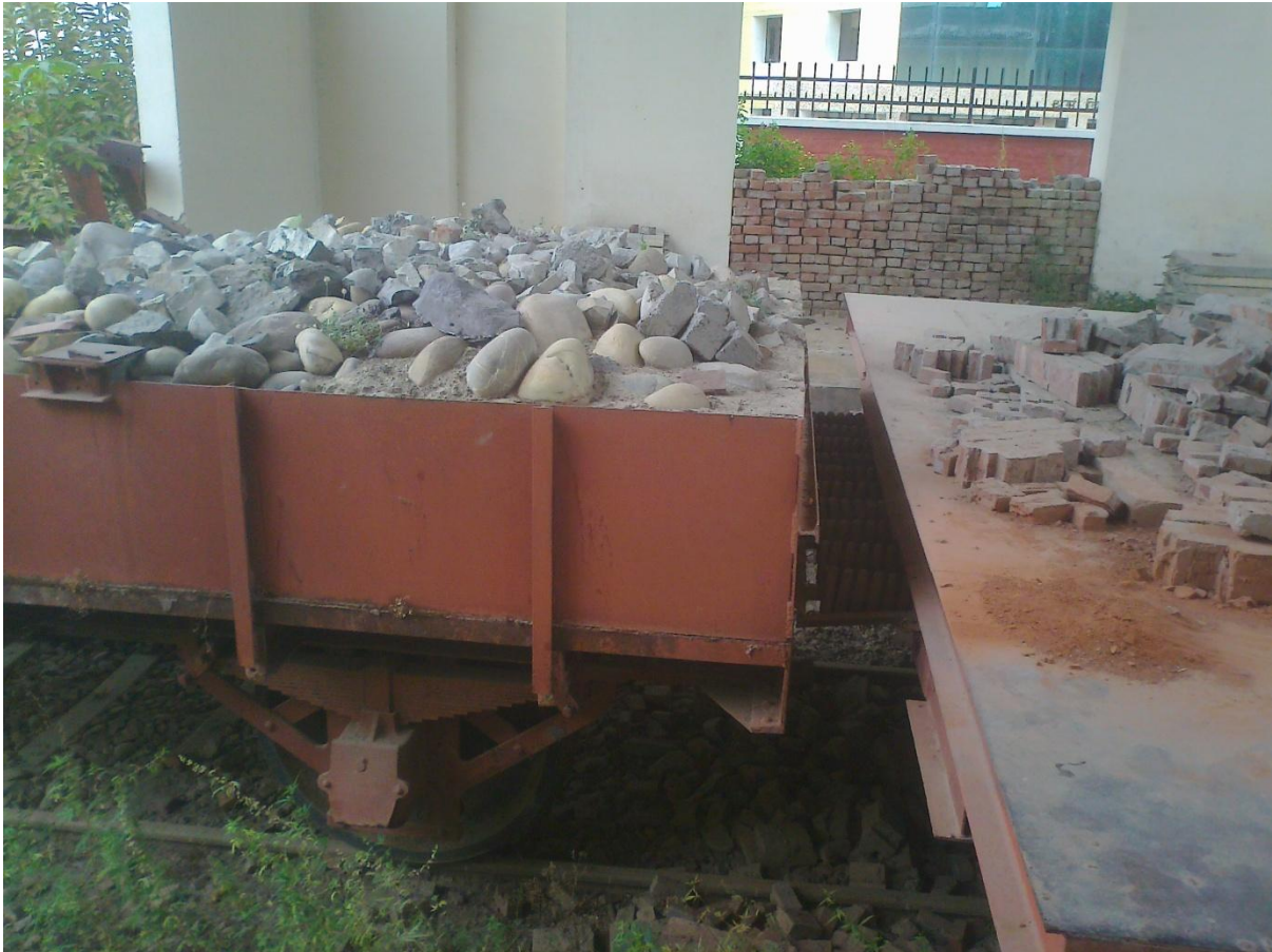
Fig.3.11: Loaded wagon hitting the Shock table platform
