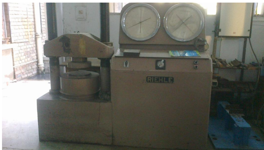
Fig.4.3: 1350 kN Compression Testing Machine (RIEHLE Instruments, AEMTEK Inc., Illinois)
