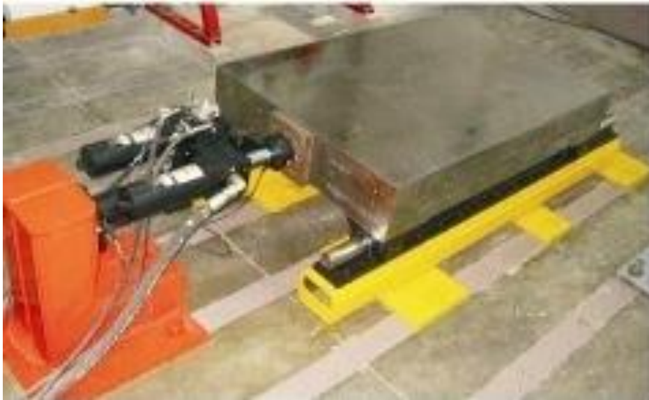
Fig.4.8: Uni-axial servo-hydraulic shake table facility
