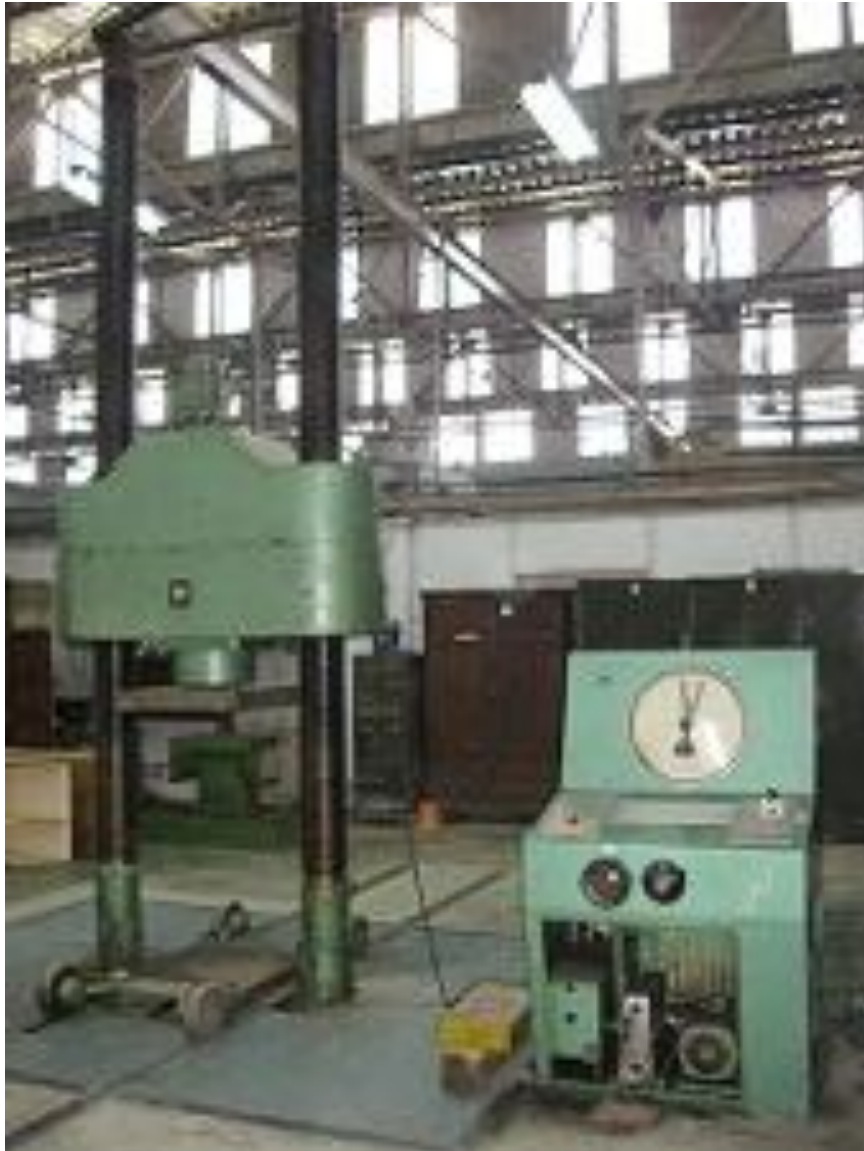
Fig.4.4: 6000kN Column Testing machine (WPM,Germany)
