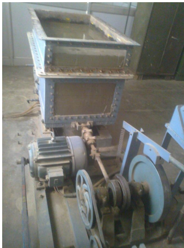
Fig.3.24: Liquefaction Table at Dept. of Earthquake Engineering, IIT Roorkee
