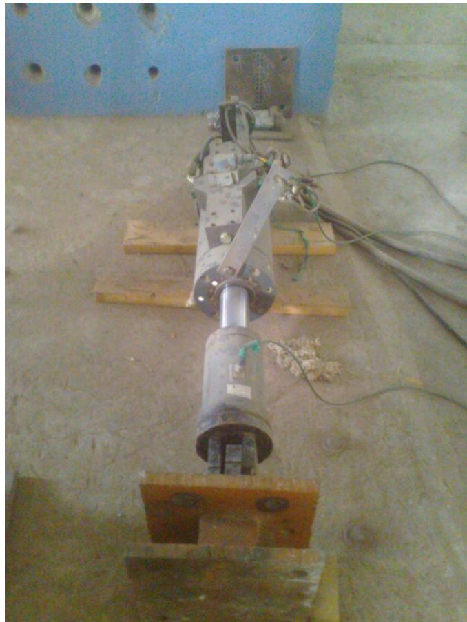
Fig.3.19 (a): Actuator (displacement based) by INSTRON
