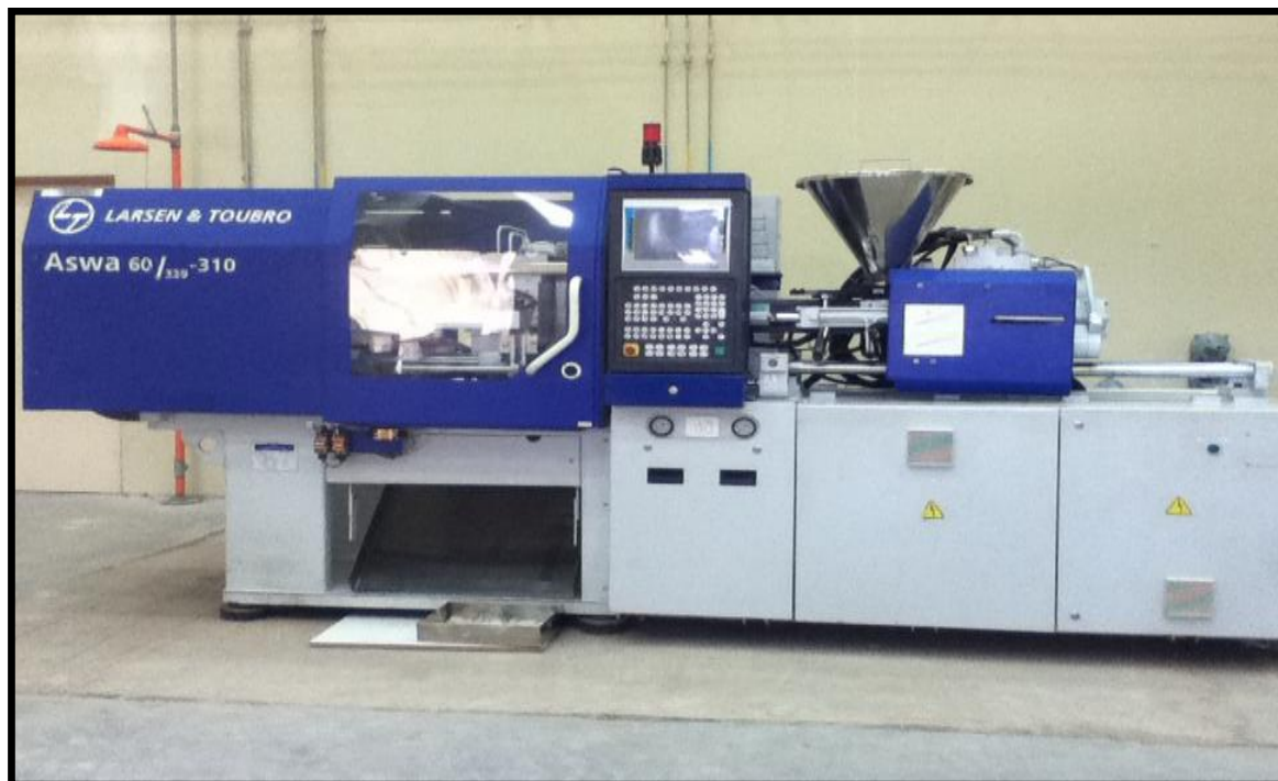
Figure 13: Injection moulding machine used for this work
