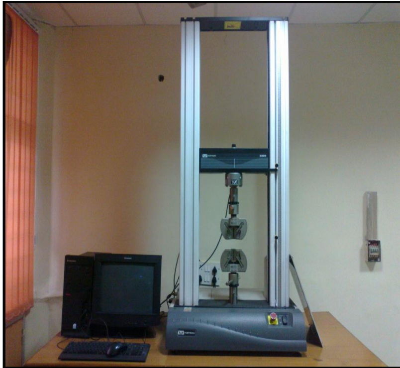
Figure 15: UTM Testing machine used for determine the tensile or flexural strength
