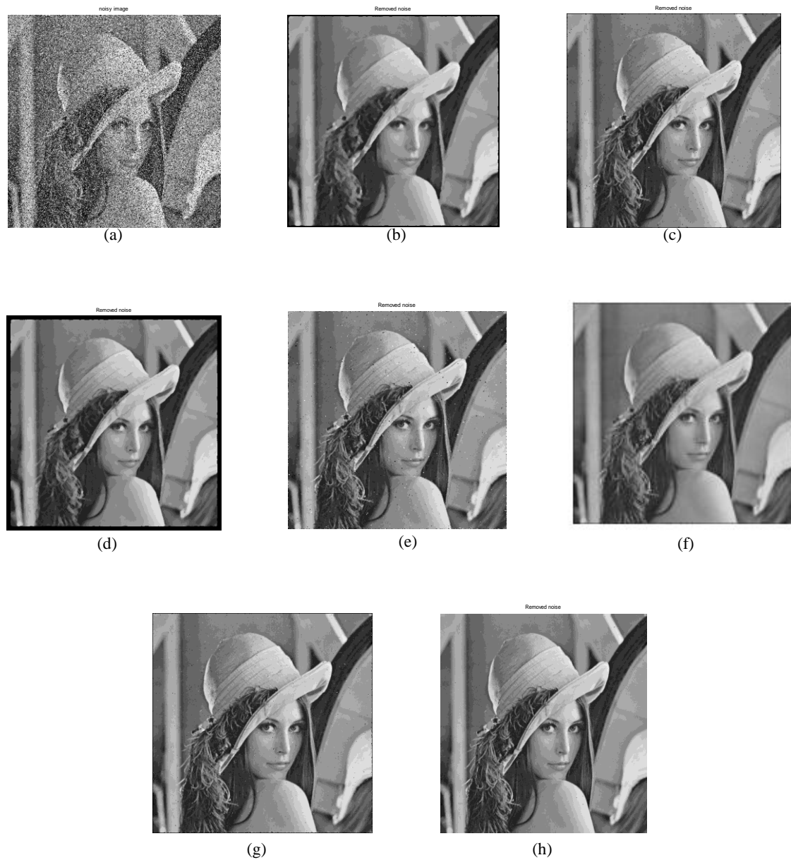
Fig 4.18: Restoration results of different methods in restoring corrupted image “Lena.” (a) corrupted image with 30% impulse noise, (b) SDOD, (c) ASWM (d) SM (e) CWM (f) CEF (g) EEPA (h) SPHN
