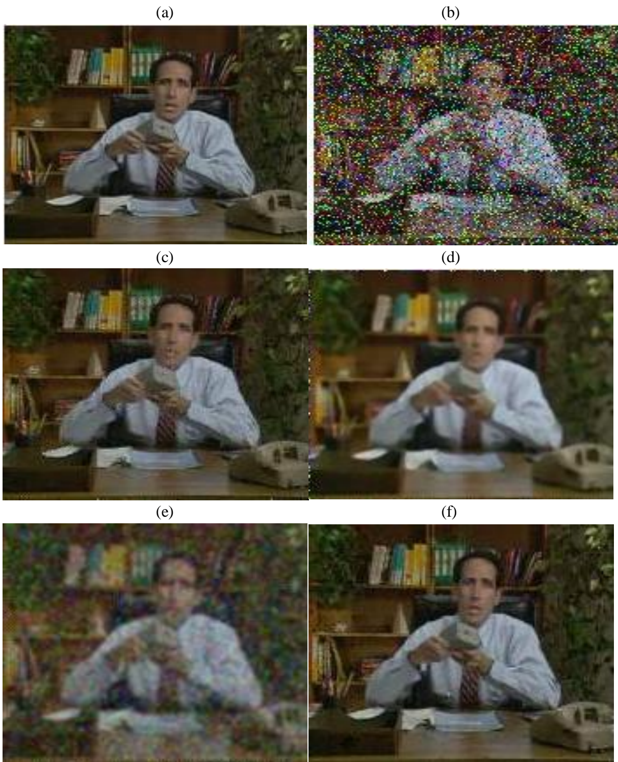
Figure 5.4: 30th frame of the “Salesman” sequence: (a) original, (b) noisy ( p=20\% ), (c) FRINRFCIS, (d) VATM, (e) KNNF and (f) Proposed.
