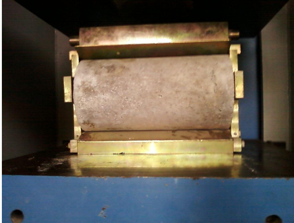
Fig. 3.2 Tensile testing of cylinder in CTM
