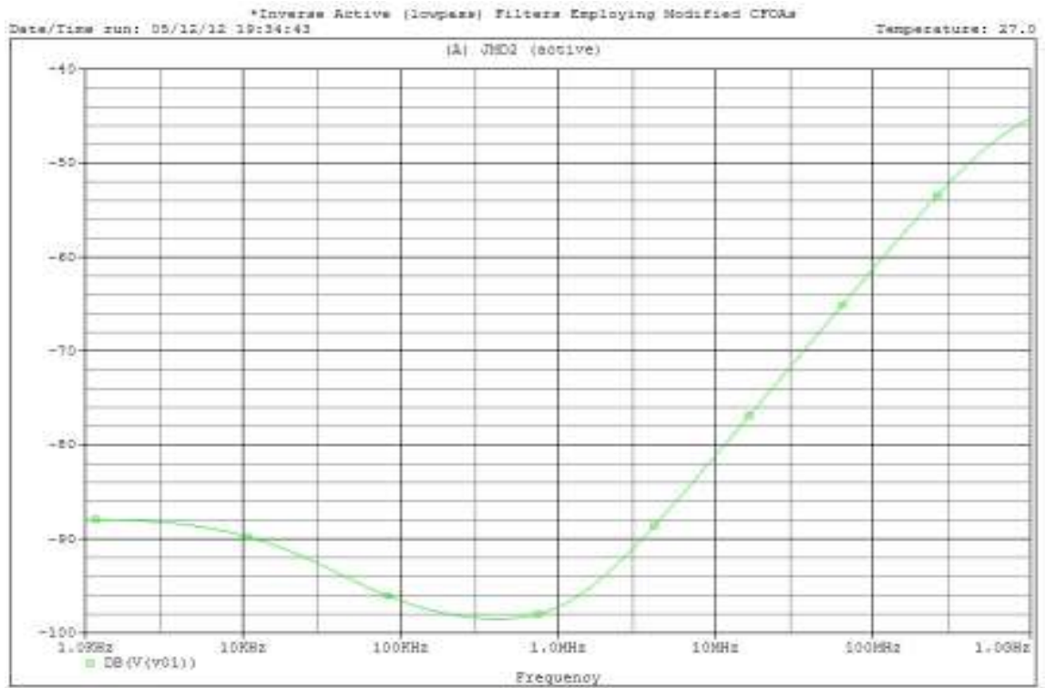
Fig.6.11: Frequency response of inverse low pass filter using Modified CFOA
