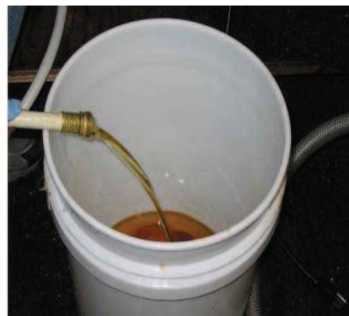
Figure 3.3: Draining biodiesel layer.
