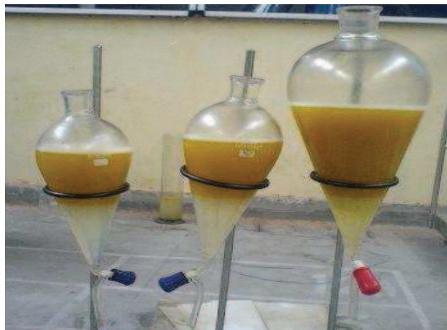
Figure 3.5: Photograph of washing process of biodiesel
