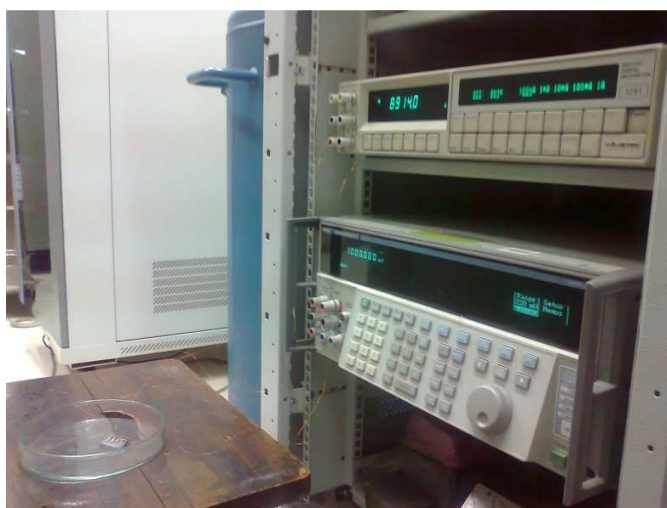
Figure 5.2 Experimental set-up for measuring I-V curve of ZnS samples
