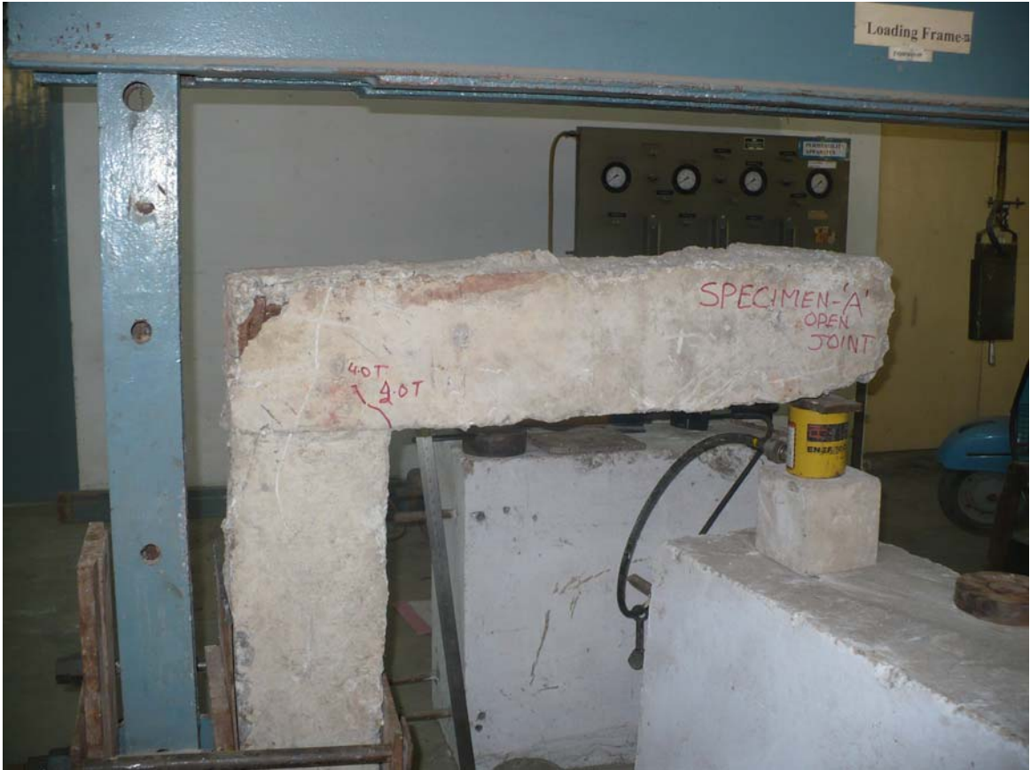
FIGURE 82: TYPE –A3 - SPECIMEN AFTER TEST-OPEN JOINT
