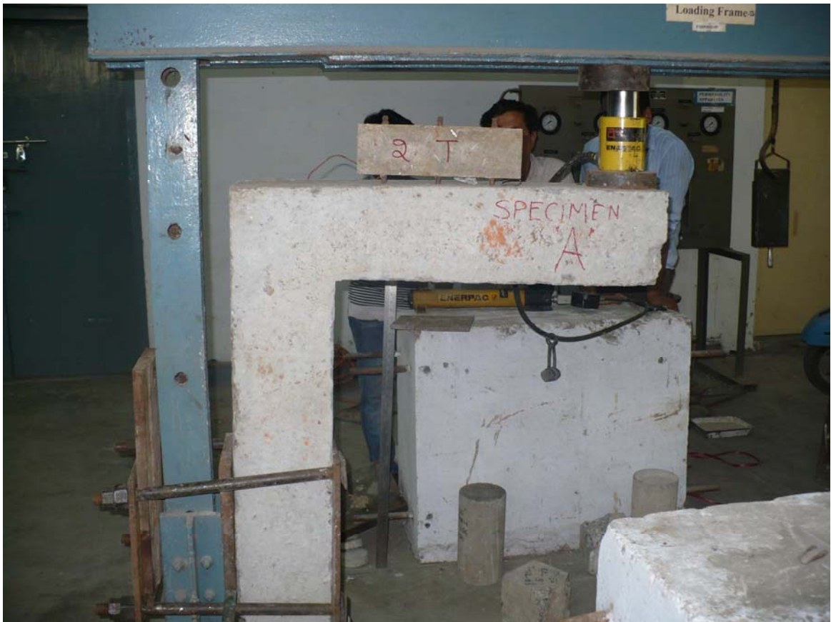
FIGURE 77: TYPE –A-SPECIMEN AFTER TEST-CLOSE JOINT
