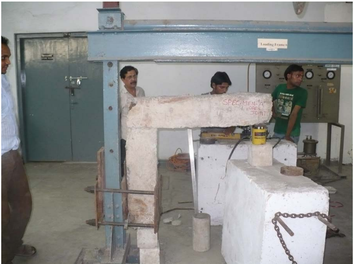
FIGURE 81: TYPE –A2--SPECIMEN AFTER TEST-OPEN JOINT
