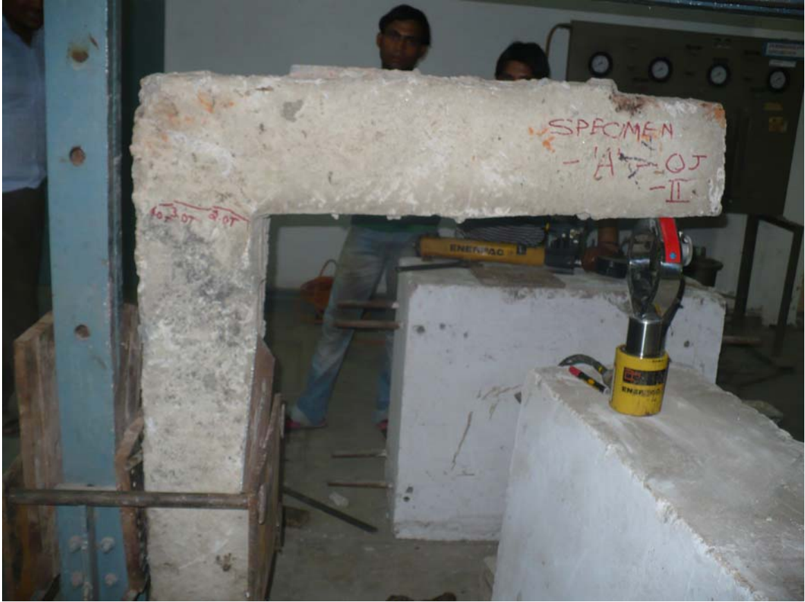
FIGURE 83: TYPE –A4-SPECIMEN AFTER TEST-OPEN JOINT
