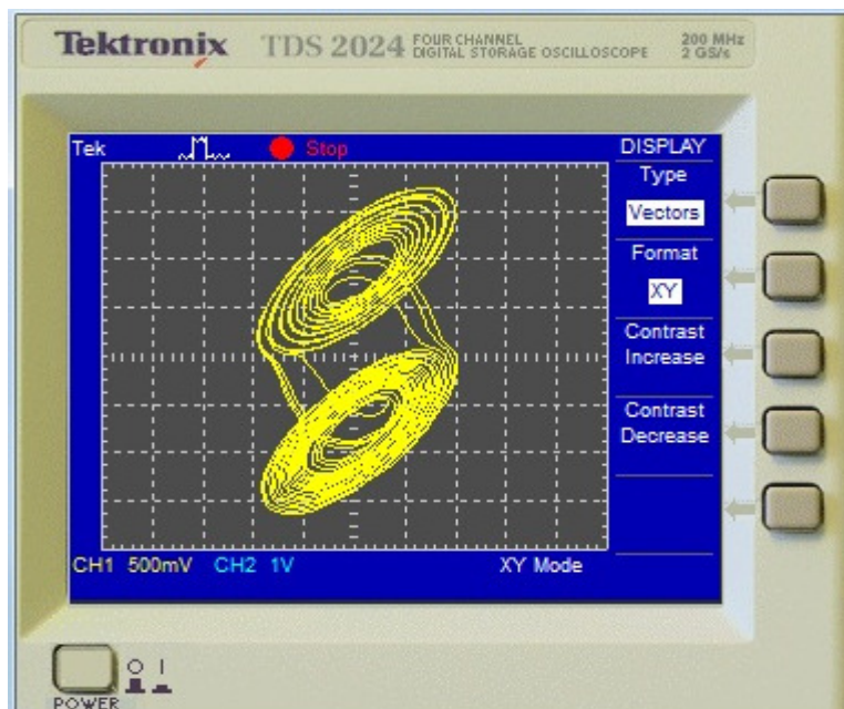
Fig.4.6. Double scroll chua's attractor with R10 equal to 1.6k ohm.
