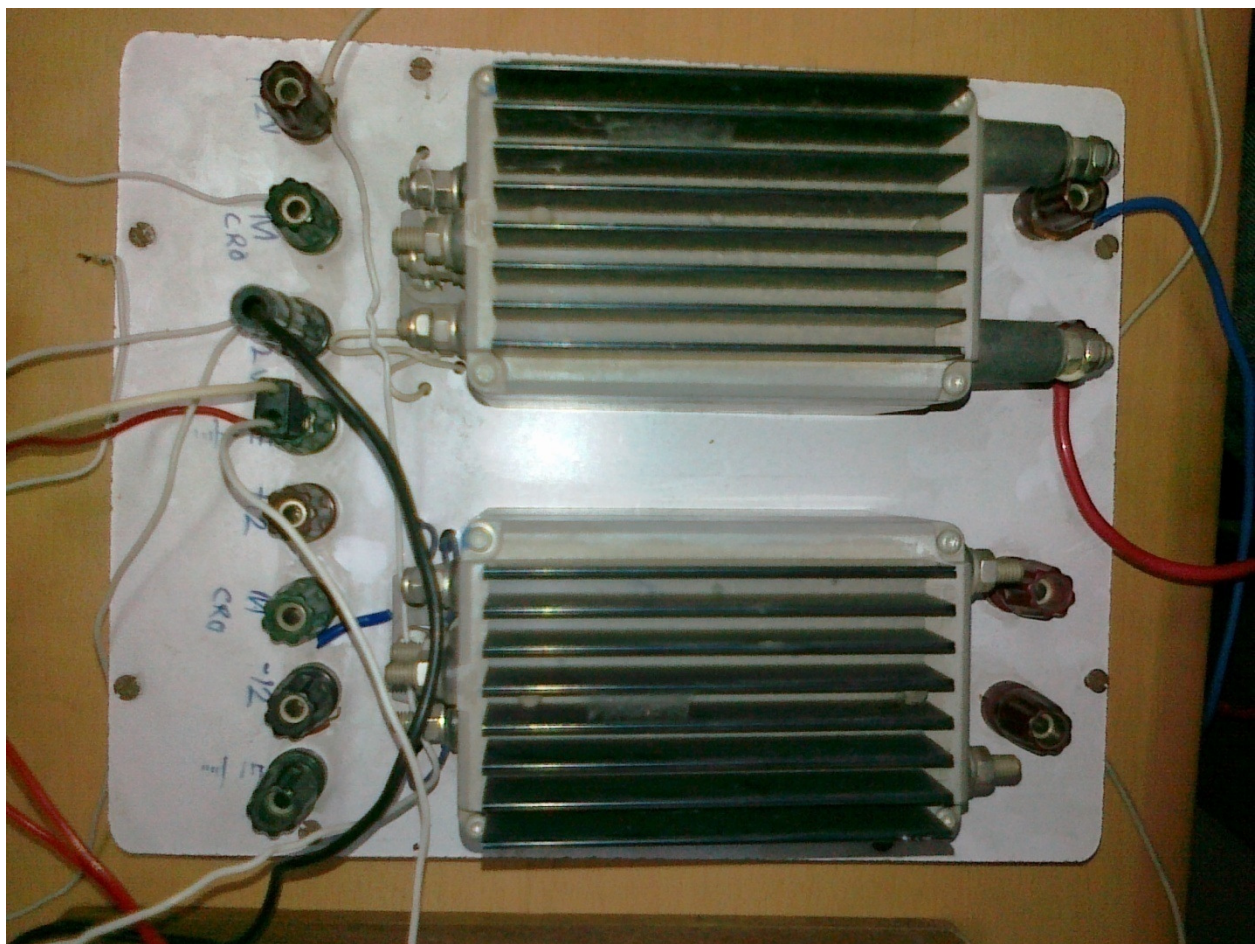
Fig 5.4 Voltage sensor with model EM010-9317 has been used in the project.
