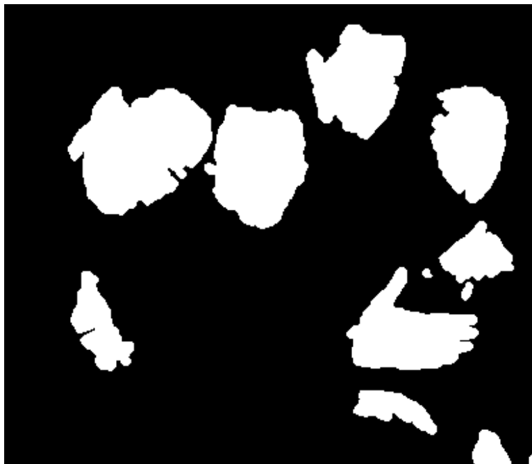
Figure 5.6: Morphological Opening Image of Disk radius 1
