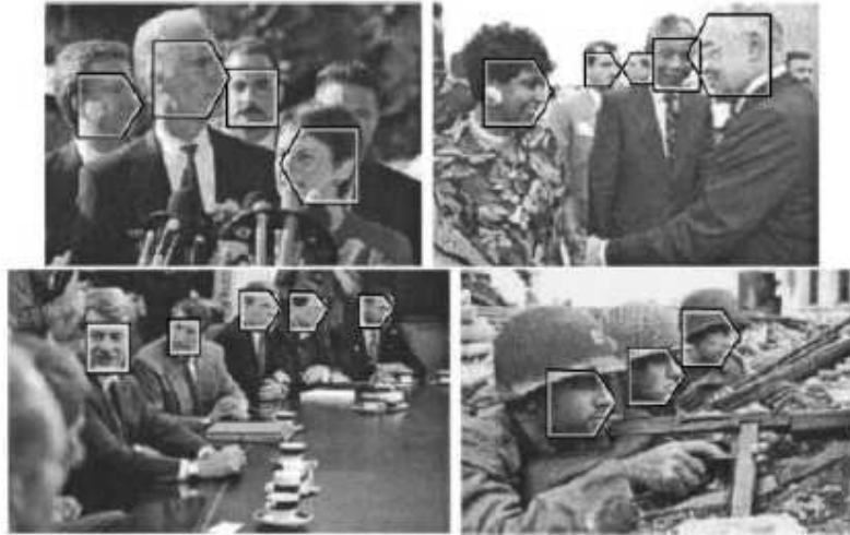
Figure 2.8: Face detection examples from Schneiderman and Kanade[6]
