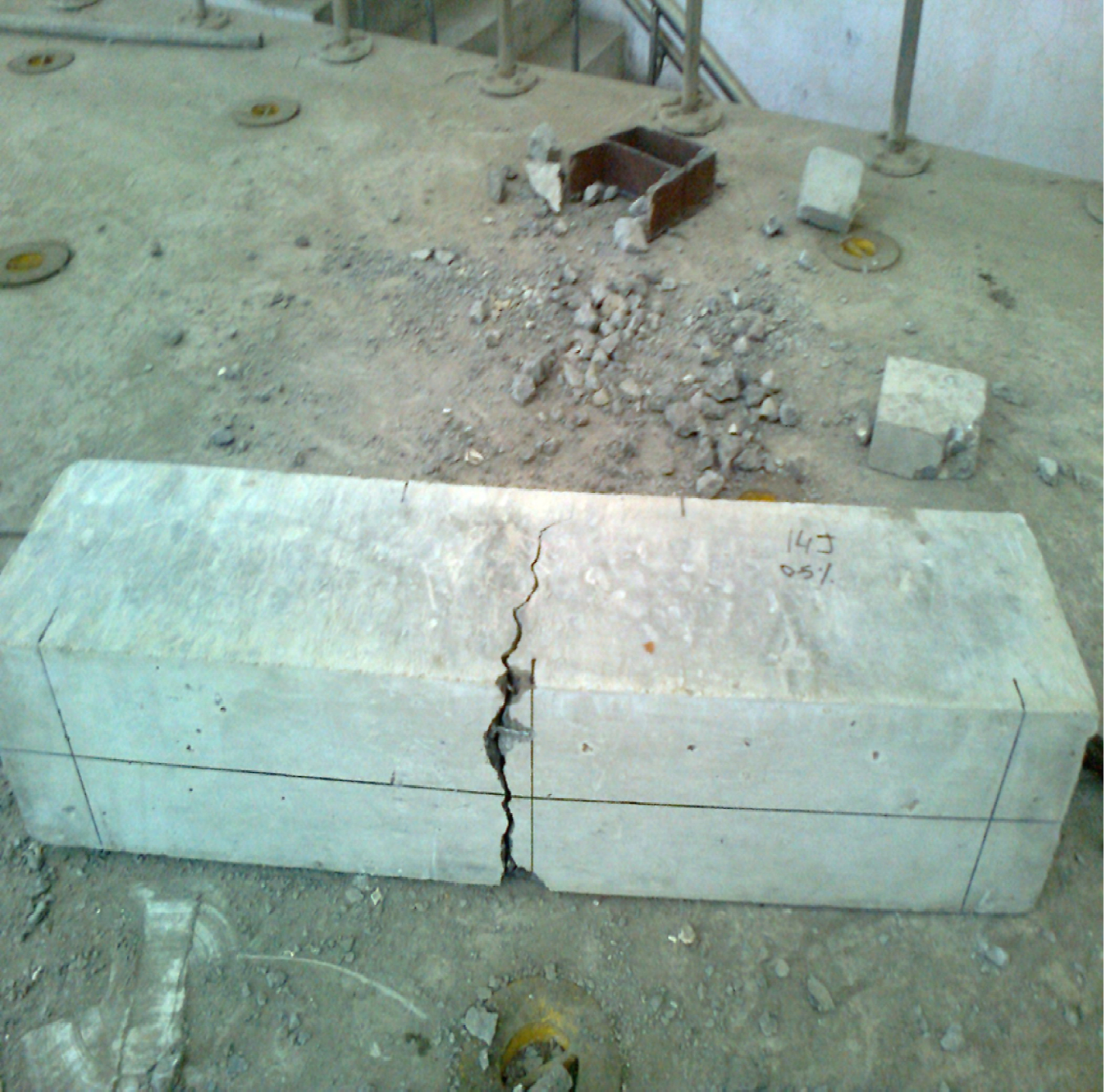
Fig 8: One of the concrete samples with 0.5% volume of steel fiber
