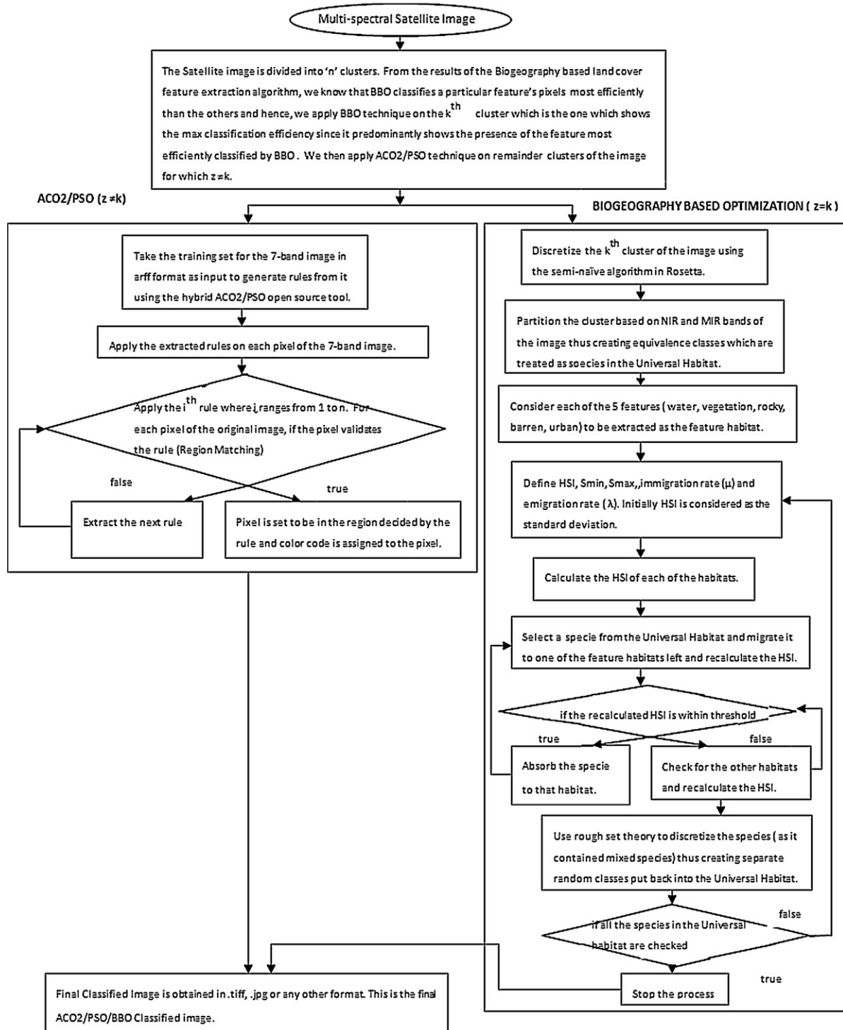
Fig. 10. Detailed Internal architecture of the Hybrid ACO2/PSO/BBO Classifier.
