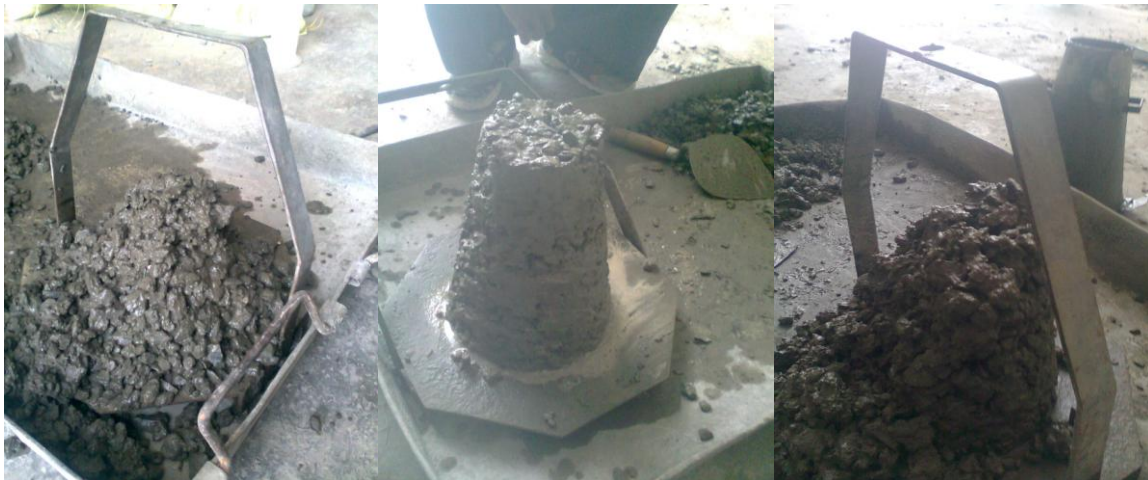
Fig. 22 Profile of obtained slump showing Collapse, Zero slump and Shear slump
