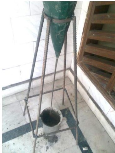
Fig 7 Cement paste flowing from Marsh cone
