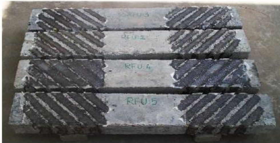
Fig 2.3 GFRP inclined U strips of various widths
