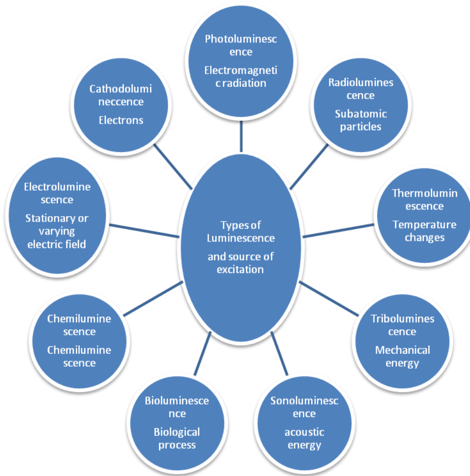
Figure 1.2 Schematic Diagram Showing types of Luminescence depending upon the source of excitation
