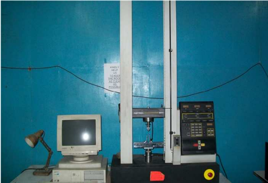
Figure 3.3: Bending Strength Instron universal testing machine
