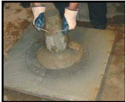
Fig. 3.3 Slump flow diameter test
