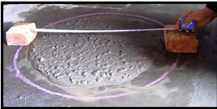
Fig3.4 T 500 Slump flow diameter test
