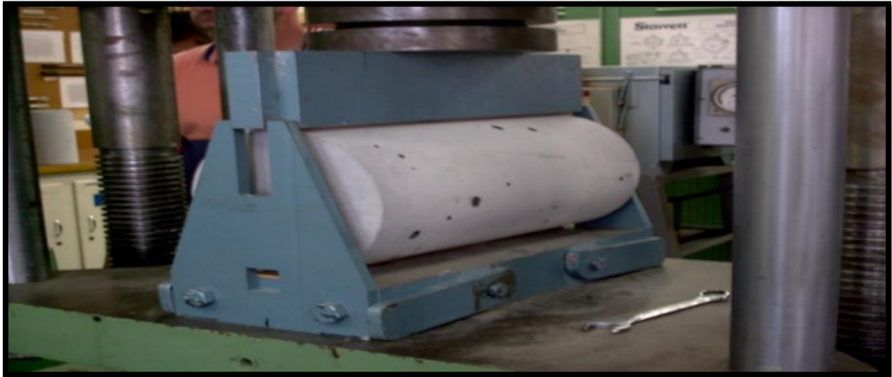
Fig. 3.9 Split tensile testing
