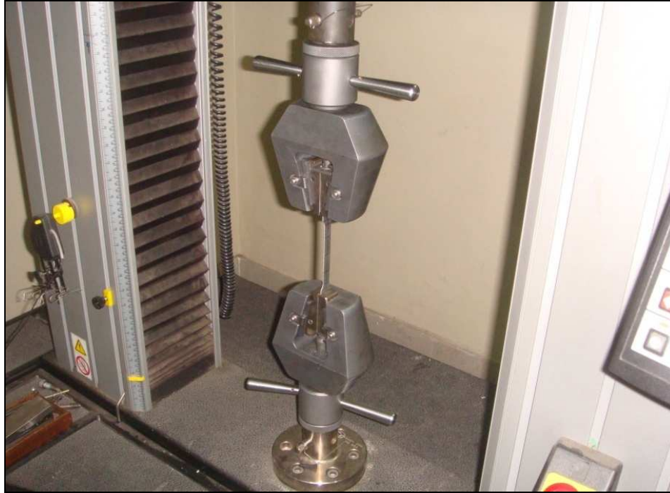
Fig. 12: 10 Ton Instron machine used for tensile testing
