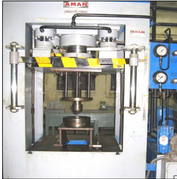
Fig. 17 Experimental setup on the 100-tonne hydraulic press
