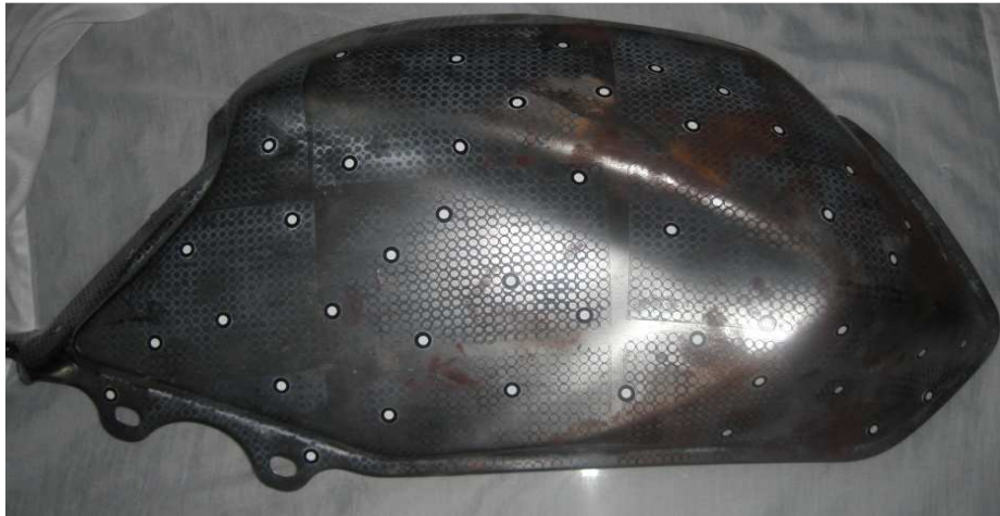
Fig . 26 Fuel tank exterior without flange
