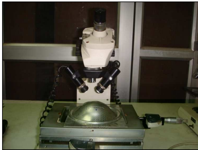
Fig 19 Travelling Microscope used for measuring deformed circles.
