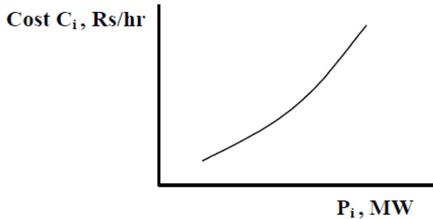
Fig 5.1(b) Fuel-rate curve
