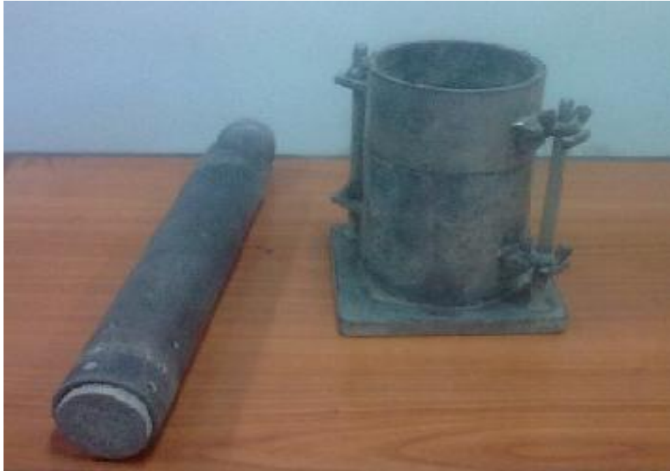
Pic. 10 - Standard Proctor Test Apparatus
