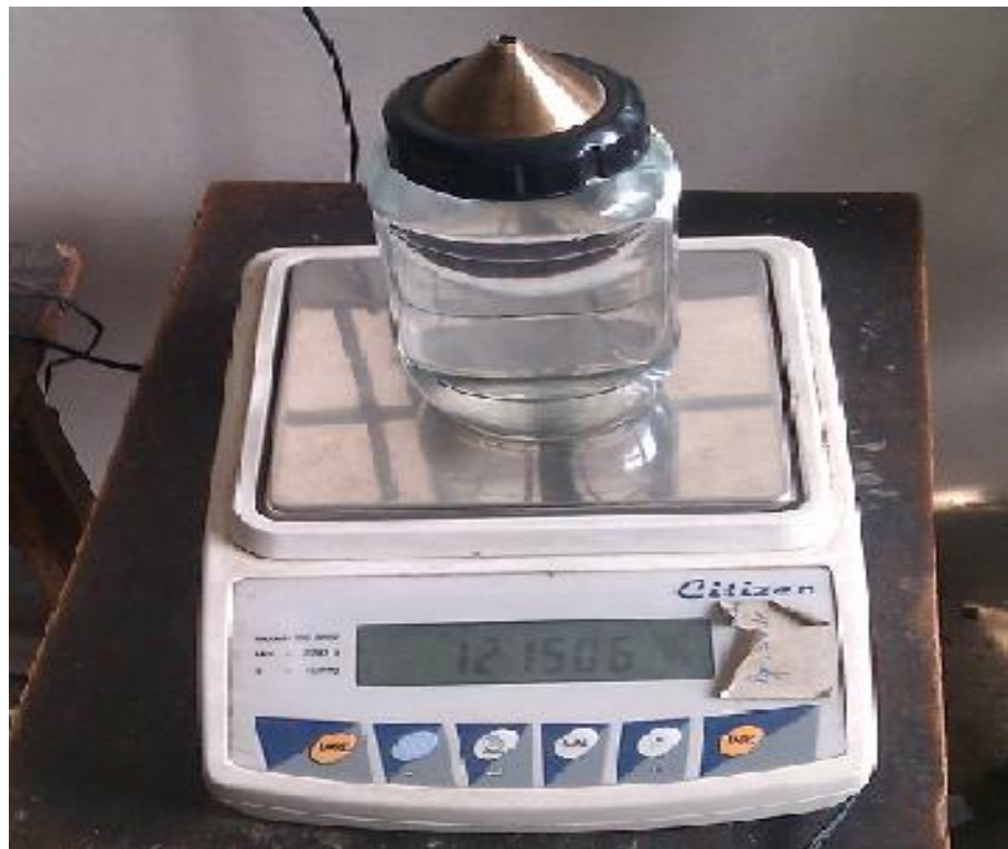
Pic. 9 - Pycnometer with water
