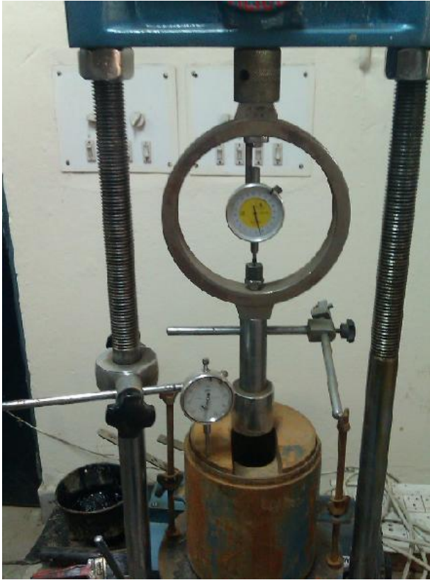
Pic. 15 - CBR Test setup
