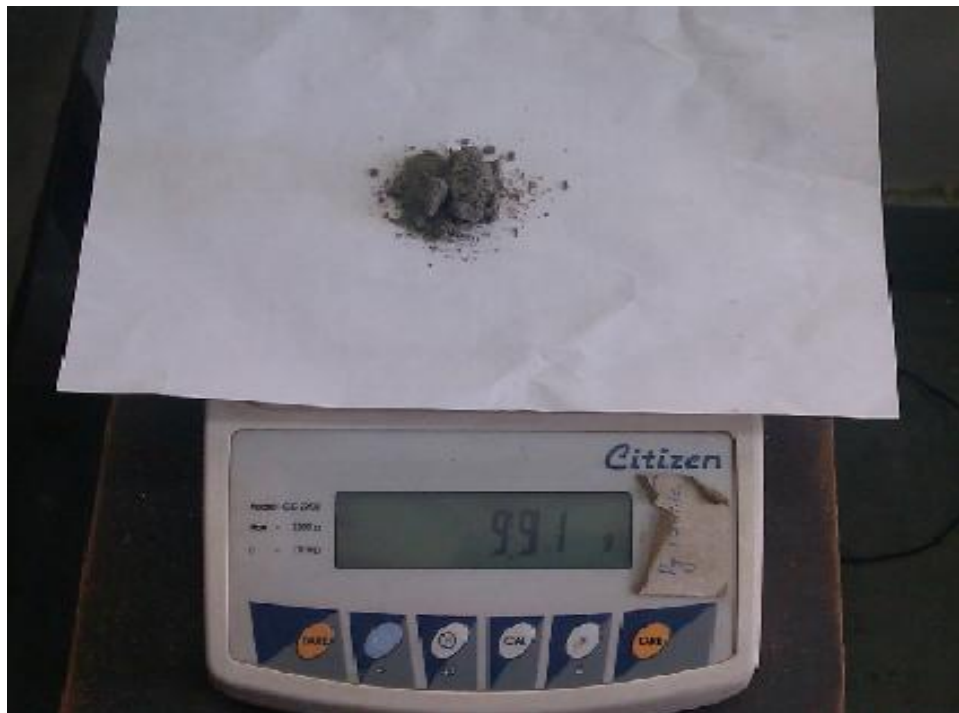
Pic. 11 - Weighing of sample to find moisture content
