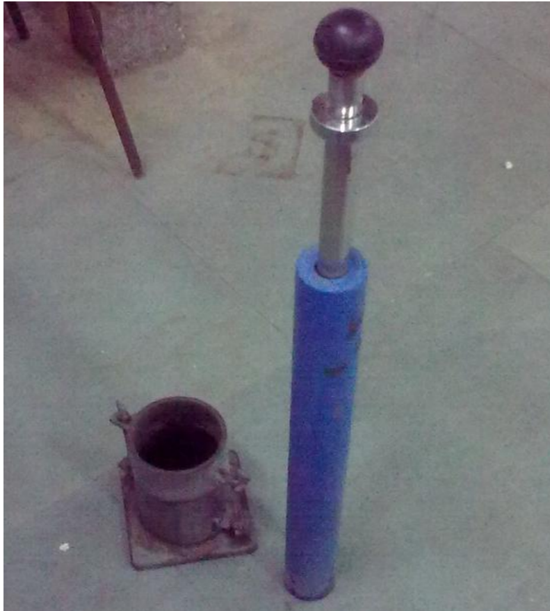
Pic. 12 - Modified Proctor Test Apparatus
