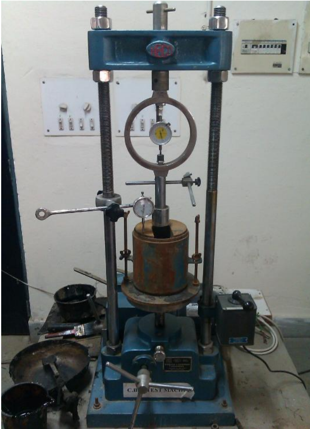
Pic. 14 - California Bearing Ratio Test Machine
