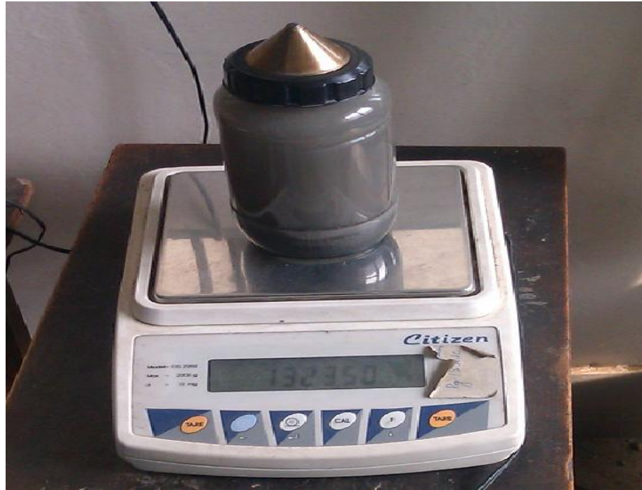
Pic. 8 - Pycnometer with water and sample
