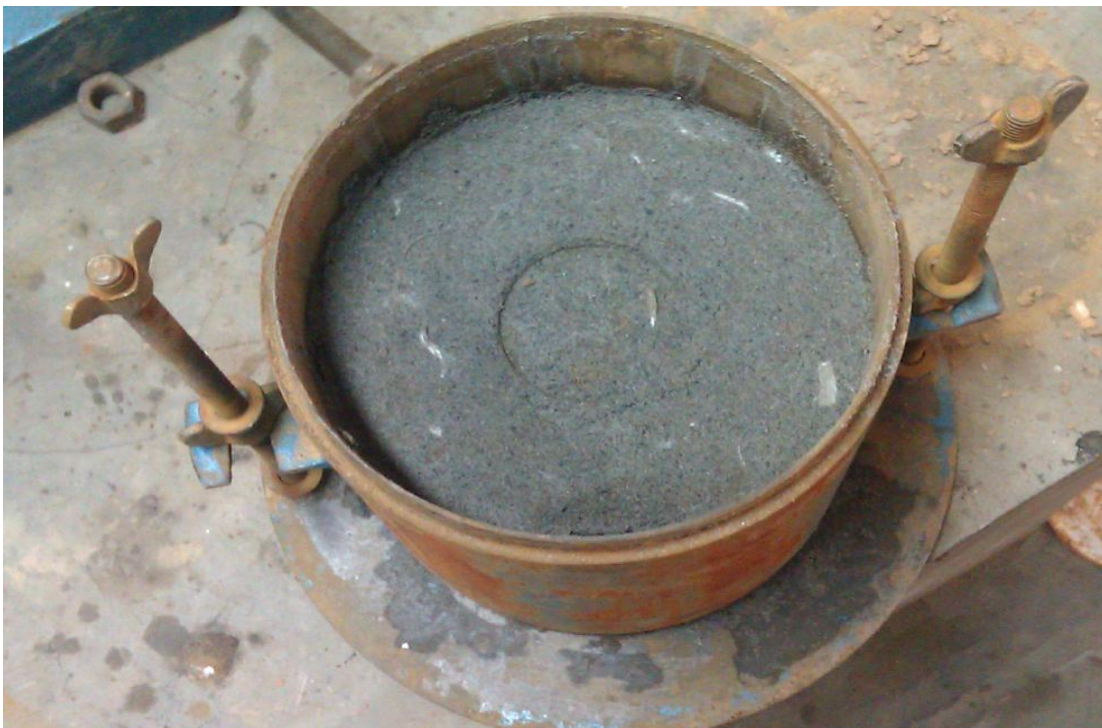
Pic. 16 - Imprint of Plunger on the sample after the test
