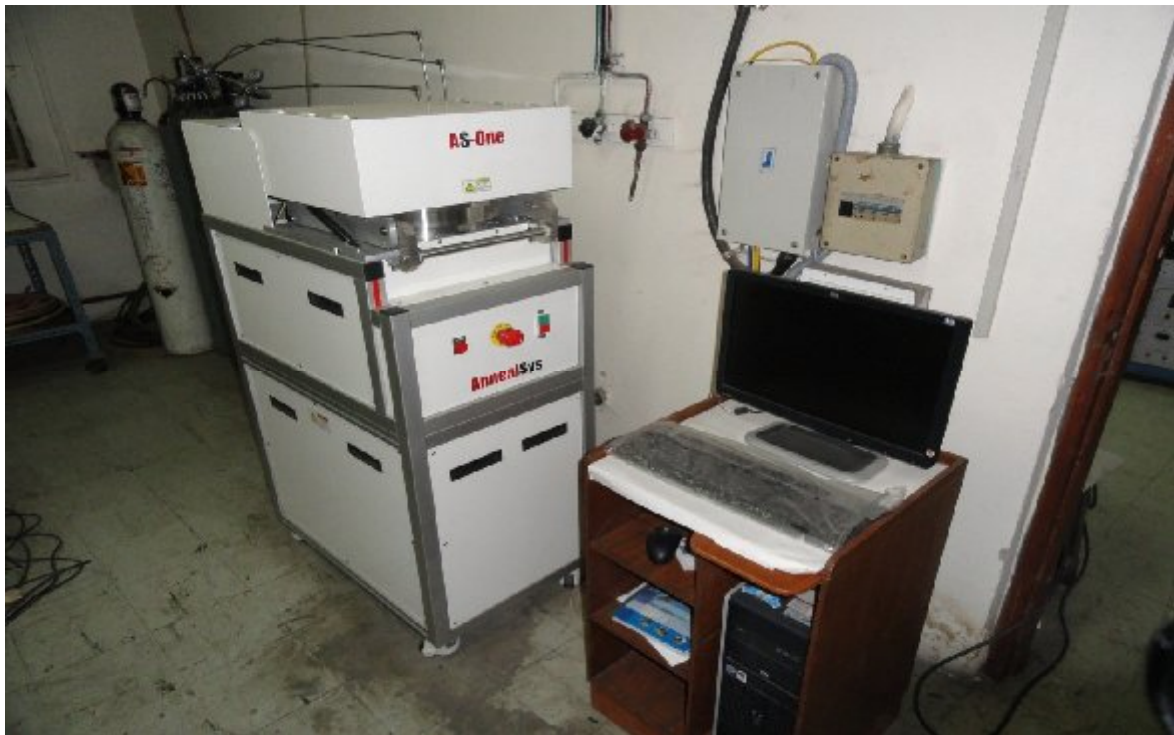
Figure 2.7: Rapid thermal processing unit for firing contacts sintering and BSF formation.
