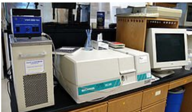
Fig 5.8 Schematic shows an UV/Vis spectrophotometer
