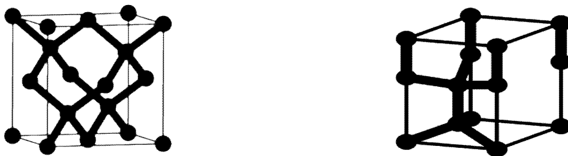
Fig 3.3 (a) Sphalerite, more common polymorph of ZnS (b) Wurtzite, less common polymorph of ZnS
