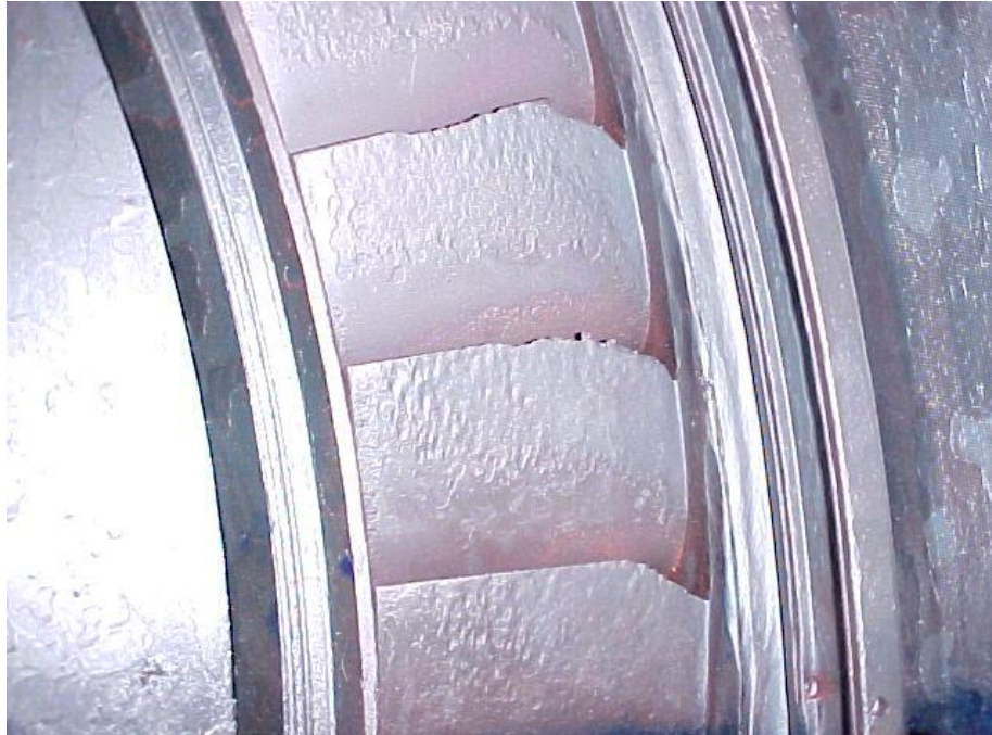
Figure 3.2 Roughness caused by solid particle erosion of turbine diaphragm (NTPC Vindhyachal).
