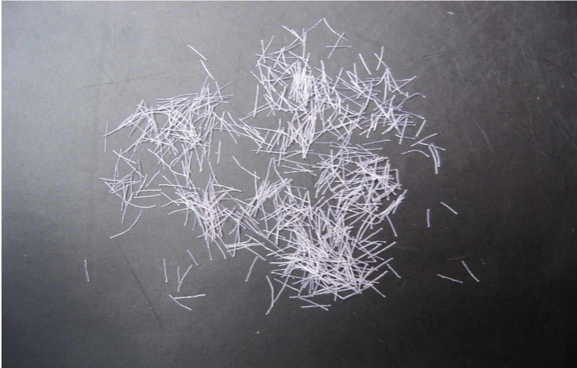
Fig 3.3:- monofilament polypropylene fibers (length=5mm)
