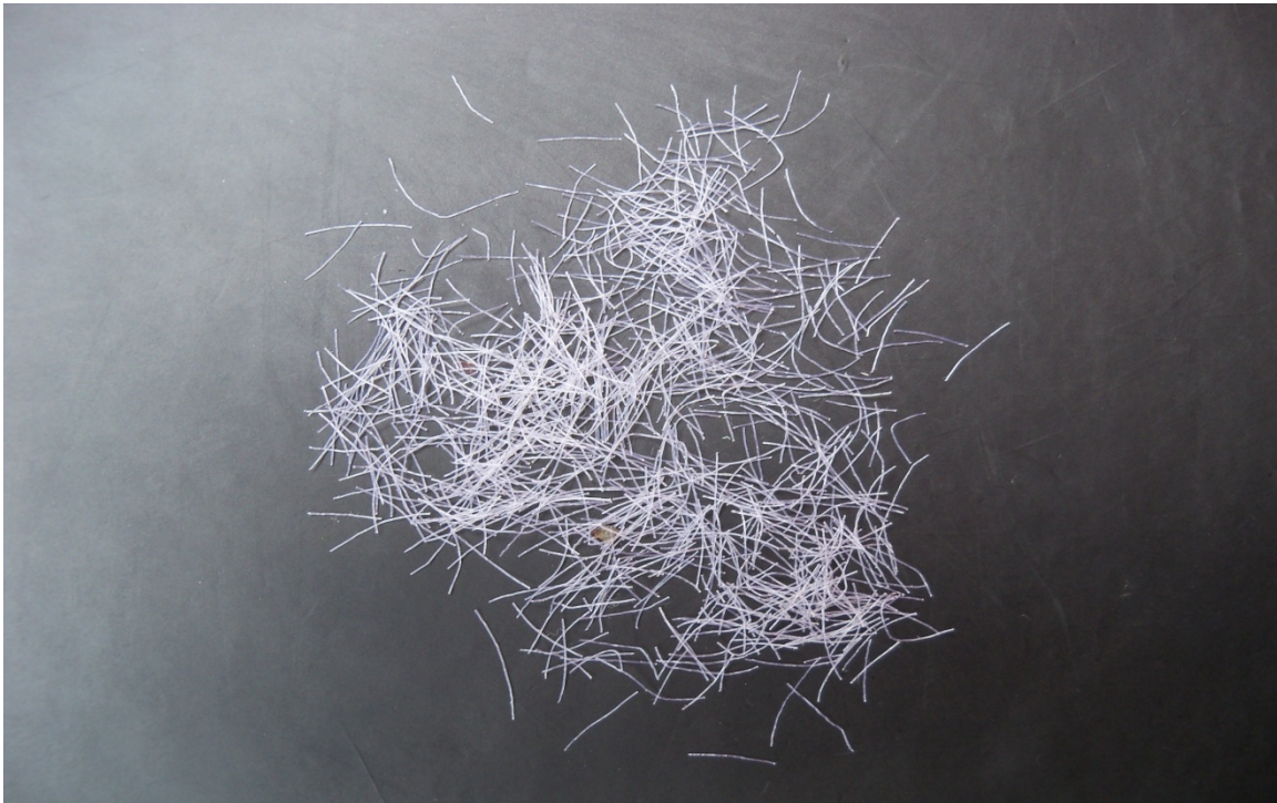
Fig 3.2 :-monofilament polypropylene fibers (length=10mm)
