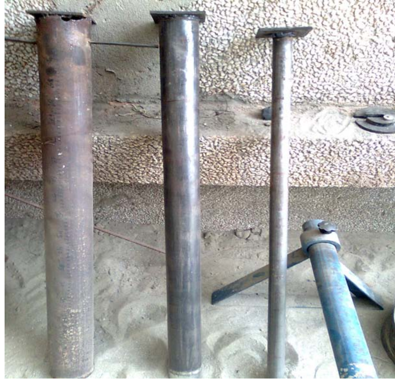
Fig 3.6:-100mm ,75mm & 40mm complete pile ready to use
