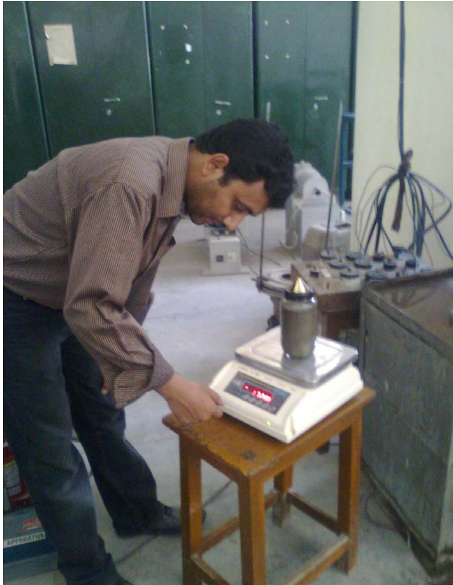
Figure 3.2:-Specific Gravity Determination By Pycnometer
