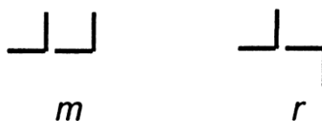
Figure 1.3: The m, meso-diad and the r, racemic diad, depending on the relative position of the CH 3 - group as described by Busico and Cipullo (2001) [11].
