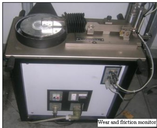
Figure 18. Wear and friction monitor machine for pin on disc test
