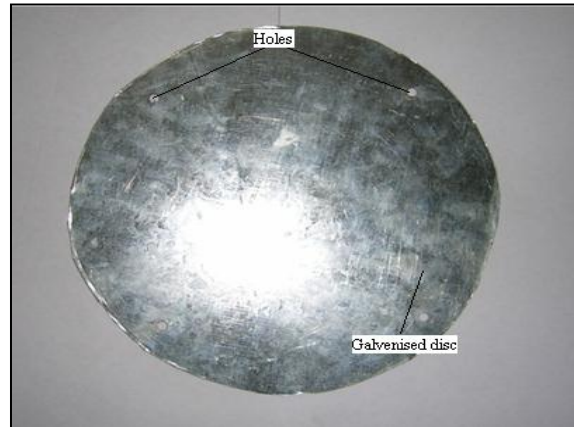
Figure 16. Galvanized disc for pin on disc test without coating
