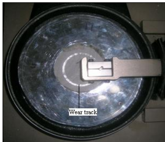
Figure 20. Thermal sprays coating during wear test
