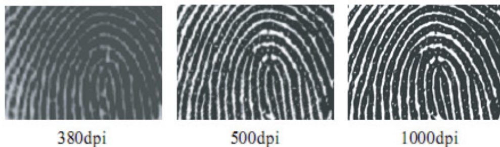
Figure 4.4 Fingerprint Features. (a) A partial fingerprint image captured at various resolutions (380dpi, 500dpi, and 1000dpi) using Identix 200DFR and CrossMatch ID1000 sensors. (b) Features extracted at different levels from the 1000dpi fingerprint in (a).
