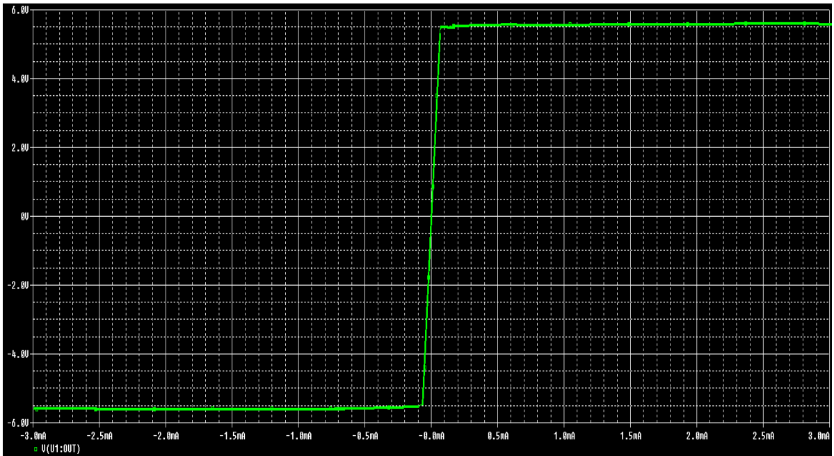
Fig. 3.5a DC characteristics of OTRA realized using CFOA
