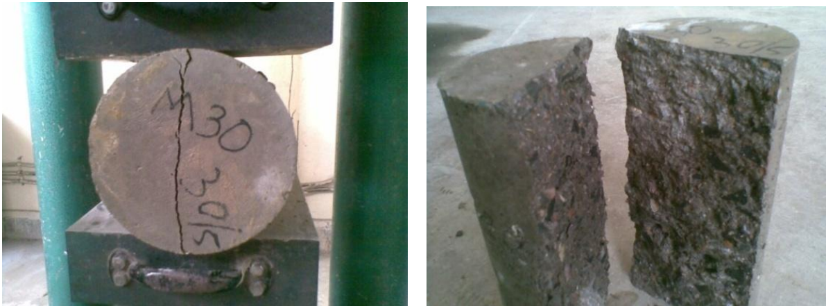
Behaviour of concrete shown after tensile test conducted
