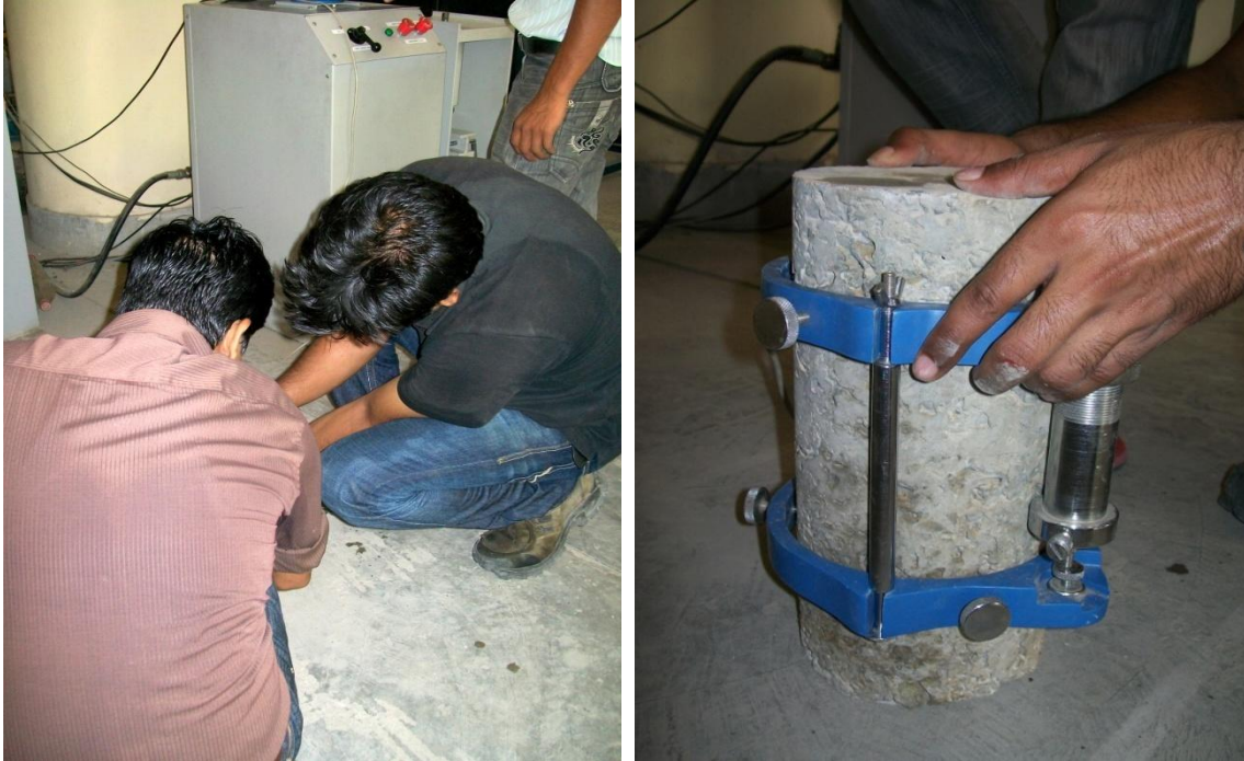
Fixing of LVDT on cylindrical specimen
