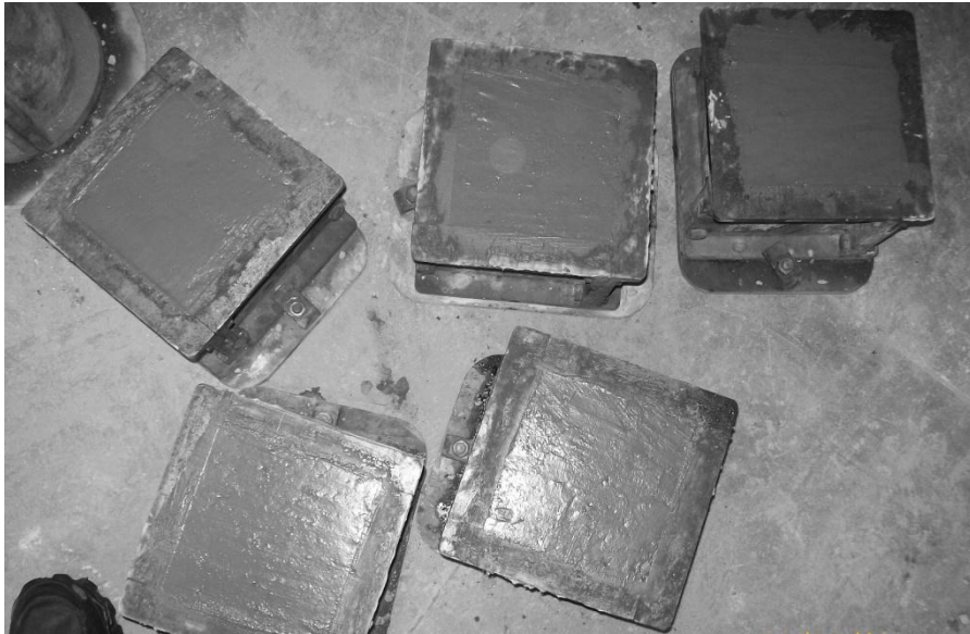
Cubical specimen casted
