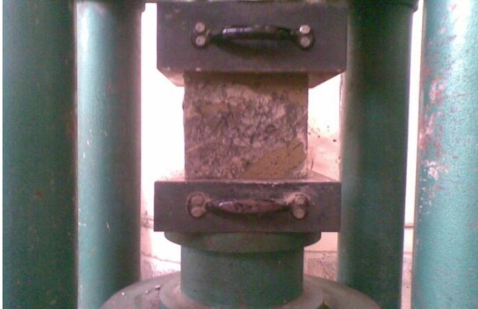
Compressive test conducted using CTM
