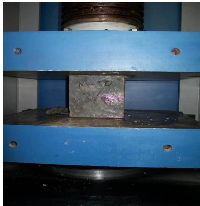
Compressive Test conducted using UTM
