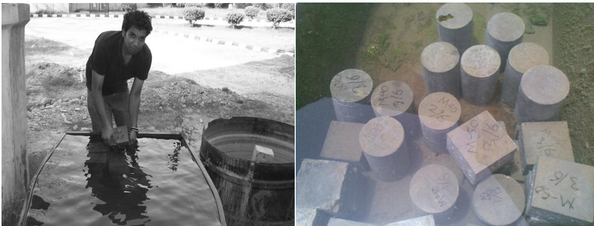
Placing of Specimens in Curing Tank after casting them
