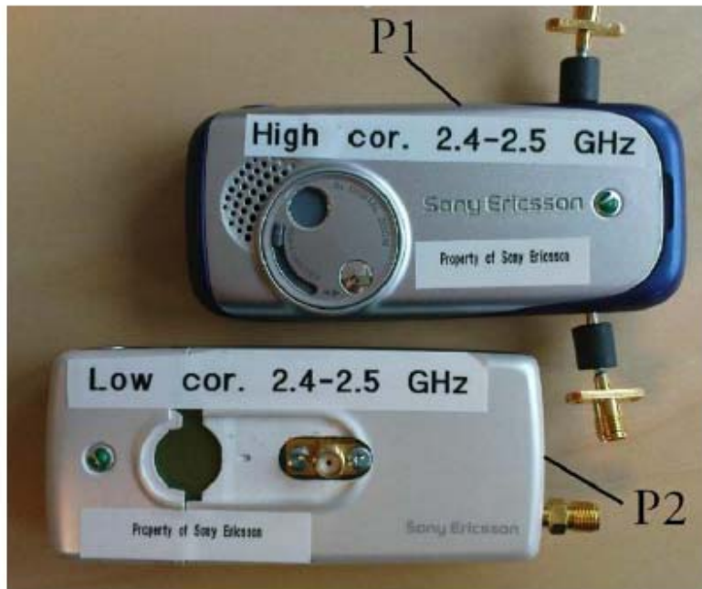
Photograph of the two terminal prototypes P1 and P2.
